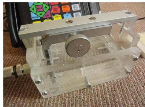
Fig. 2. Measurement tank and the sample holder and positioning system.
