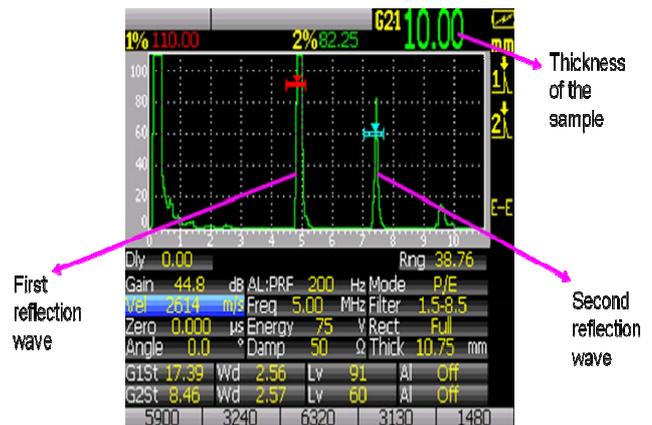
Fig. 3. EPOCH XT screen and signification of the values.
