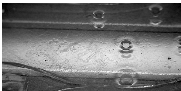
Fig. 1. Holes in the cladding surface because of a high viscosity of the Ormoclad and a not well cleaned wafer.
