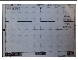
Fig.8. PWM signal of the smart lighting system Case 2
