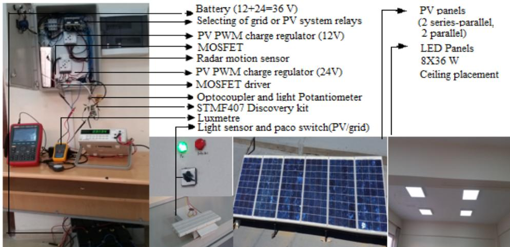
Fig. 4. PV-based smart LED illuminating system.
