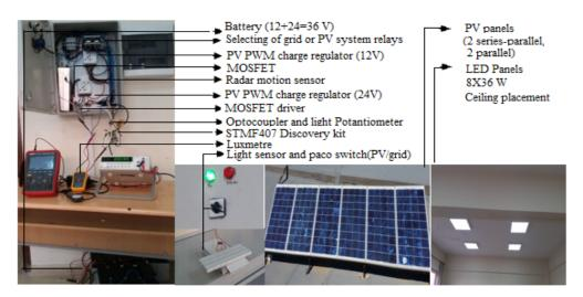
Fig. 4. PV-based smart LED illuminating system.
