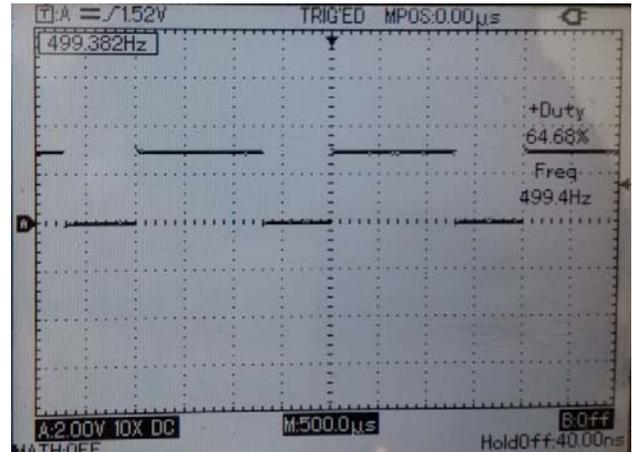
Fig.8. PWM signal of the smart lighting system Case 2
