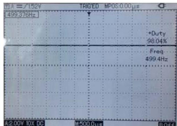
Fig. 9. PWM signal of the smart lighting system Case 3
