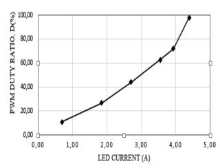
Fig.10. Measured LED panels current over the duty ratio of the PWM signals in proposed lighting system.
