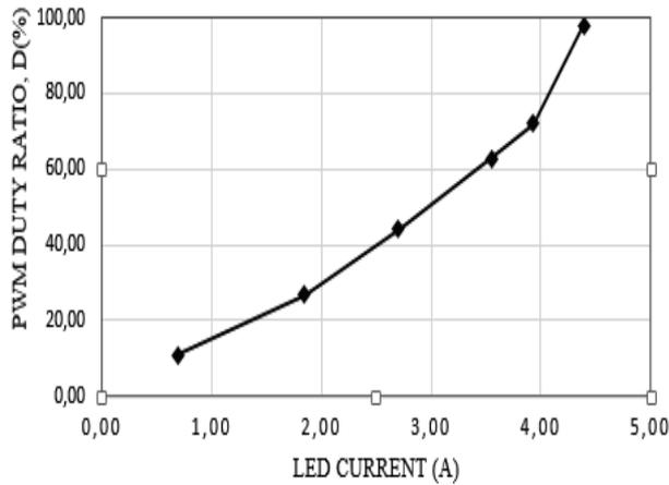
Fig.10. Measured LED panels current over the duty ratio of the PWM signals in proposed lighting system.
