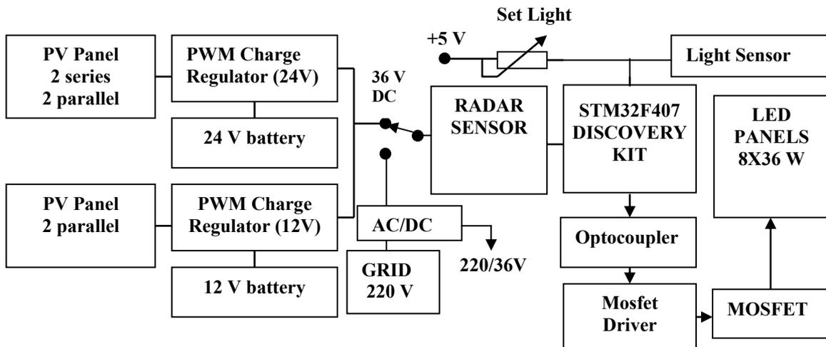
Fig. 5. PV-based smart LED illuminating system block chart
