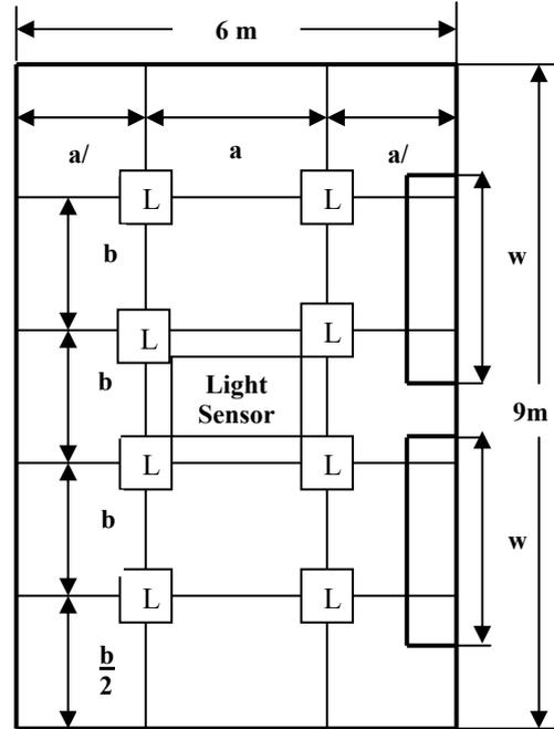
Fig. 3. Layout of LED panels and Light Sensor on Ceiling
