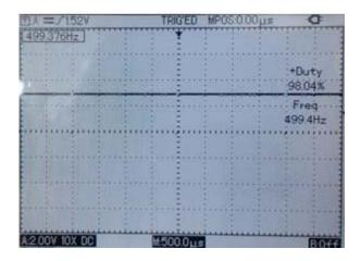
Fig. 9. PWM signal of the smart lighting system Case 3
