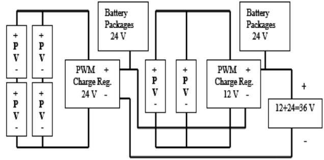
Fig.2. PV panels DC system composed of charge regulators
