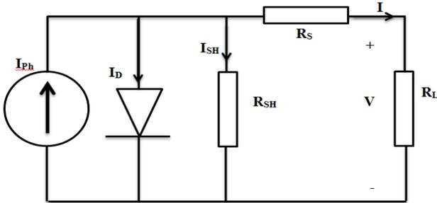
Fig. 1. Equivalent circuit diagram for solar cells
