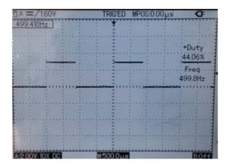
Fig.7. PWM signal of the smart lighting system Case 1
