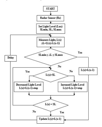
Fig. 6. Flowchart for Proposed Smart Control Algorithm
