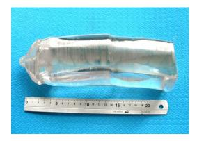
Fig. 2. ZnWO<sub>4</sub> crystal grown by LTG Cz technique (NIIC SIB RAS, Novosibirsk)
