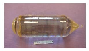
Fig. 1. CdWO<sub>4</sub> crystal grown by LTG Cz technique (CML ltd, Novosibirsk)
