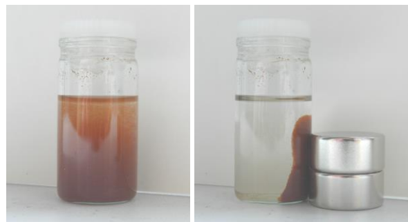
Fig. 7. The magnetic polymer particles suspension in acetone, in absence (first image) and in presence (second image) of magnetic external field (produced by high force magnets).
