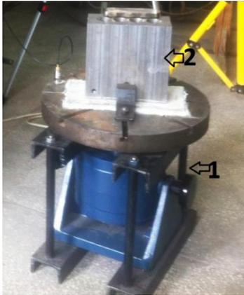
Fig. 1. Setup of the electrodynamic exciter (1) and metallic mould (2).
