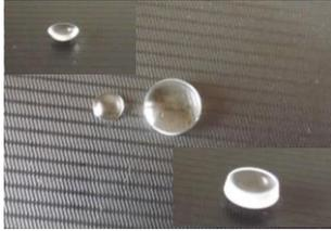
Fig. 13. Photos of the meniscus and the bi-convex lenses, the smaller one (diameter  $\sim 6$  mm) is the meniscus lens and the bigger one is the bi-convex lens (diameter  $\sim 12$  mm)
