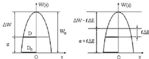
Fig. 3 The parabolic potential barrier
