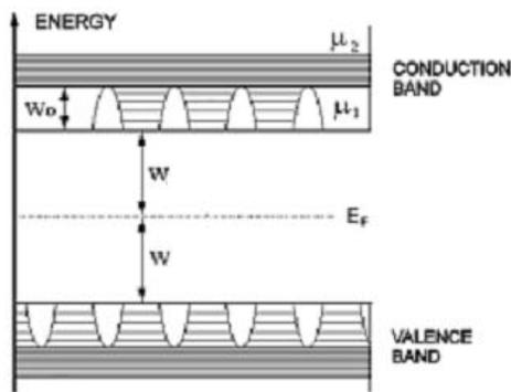
Fig. 1 Electronic spectrum of chalcogenide glass
