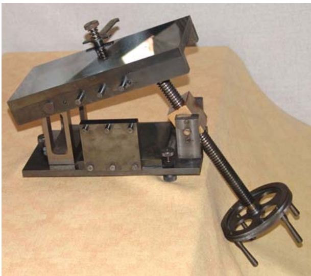
Fig. 1. Tribometer used for friction test
