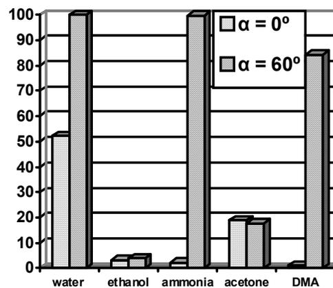
Fig. 6. Relative sensitivity  $|S|$  of AgCl films deposited at vapour incidence angles of  $0^\circ$  and  $60^\circ$  in different ambient atmospheres.
