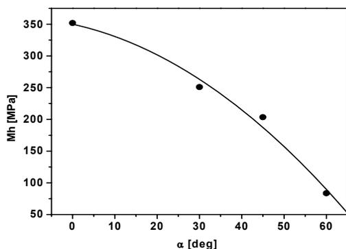
Fig. 3. Microhardness  $M_h$  of AgCl films vs. the vapour incidence angle  $\alpha$ .
