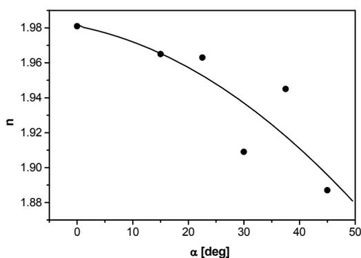
Fig. 4. Refractive index of AgCl films vs. the vapour incidence angle  $\alpha$ , calculated for  $\lambda=600$  nm.
