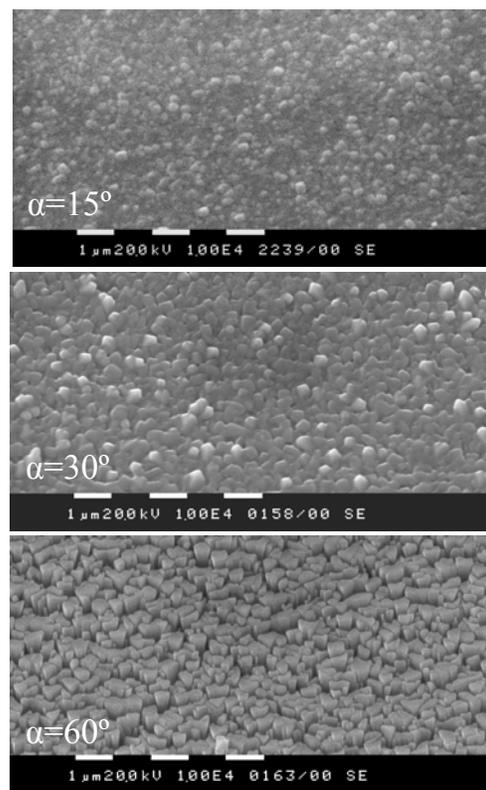
Fig. 1. SEM micrographs of AgCl films deposited at different vapour incidence angles,  $\alpha$ .
