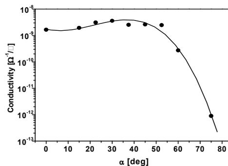
Fig. 5. DC-conductivity  $\sigma$  of AgCl films vs. the vapour incidence angle  $\alpha$  for ambient conditions ( $t=25^\circ\text{C}$ ).
