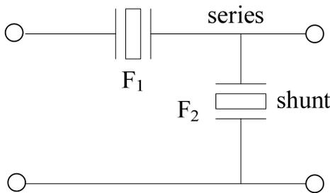
Fig. 6. Single stage Ladder-Type Filter.
