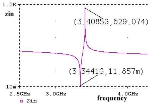
Fig. 7. The magnitude of FBAR impedance.
