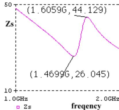
Fig. 11. The magnitude of series FBAR impedance versus frequency.
