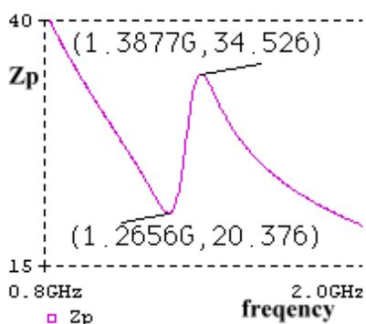
Fig. 12. The magnitude of shunt FBAR impedance versus frequency.
