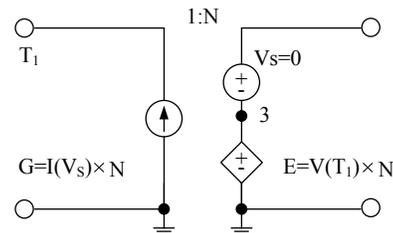
Fig. 4. PSPICE model of electromechanical transformation circuit.
