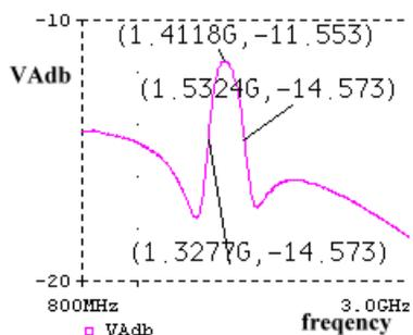
Fig. 13. The transmission transform function (TTF) of single stage ladder-type filter.
