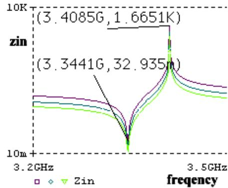
Fig. 10. Impedances of FBAR with different electromechanical factors.
