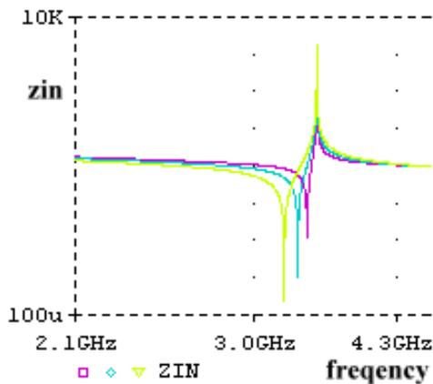
Fig. 9. The magnitude of FBAR impedance versus frequency with different electromechanical factors.
