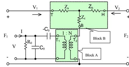
Fig. 2. Mason circuit of piezoelectric film vibrating in thickness mode.
