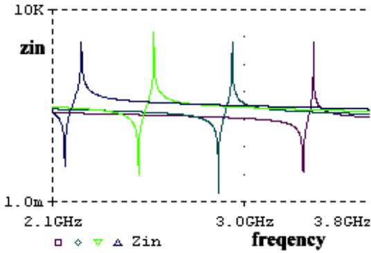
Fig. 8. The magnitude of FBAR impedance versus frequency with different thickness of piezo-film.
