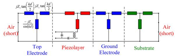
Fig. 3. Mason equivalent circuit of FBAR.
