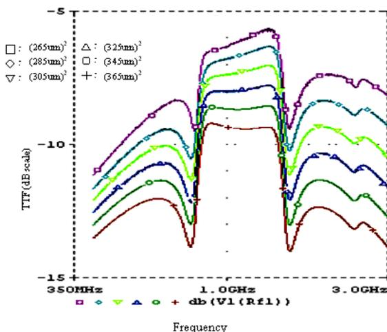
Fig. 15. The transmission transform function of two stages ladder-type filter by varying the piezo-film thickness as  $(265\mu\text{m})^2$ ,  $(285\mu\text{m})^2$ ,  $(305\mu\text{m})^2$ ,  $(325\mu\text{m})^2$ ,  $(345\mu\text{m})^2$  and  $(365\mu\text{m})^2$ , respectively.
