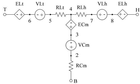
Fig. 5. PSPICE model of acoustical transmission.
