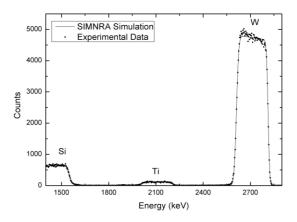
Fig. 3b. 3.065 MeV <sup>4</sup>He<sup>2+</sup> backscattered at 165° from a single layer structure of TixNy+TixByNz+WxCyNz on silicon, sample no. 2. Dots: Experimental data; Solid line: Simulation.
