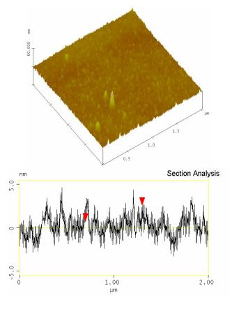
Fig. 1c. TM-AFM images showing 3D surface topography,  $2x2 \ \mu m^2$  and section analysis, sample no. 3
