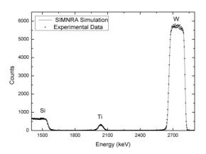
Fig. 3a. 3.065 MeV  ${}^{4}He^{2+}$  backscattered at 165 ° from a three layer structure of  $Ti_xN_y/Ti_xB_yN_z/W_xC_yN_z$  on silicon, sample no. 1. Dots: Experimental data; Solid line: Simulation.
