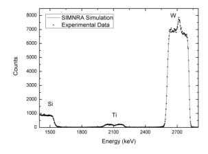
Fig. 3c. 3.065 MeV  ${}^{4}He^{2+}$  backscattered at 165 ° from a single layer structure of Ti+TiB<sub>2</sub>+WC on silicon, sample no. 3. Dots: Experimental data; Solid line: Simulation.
