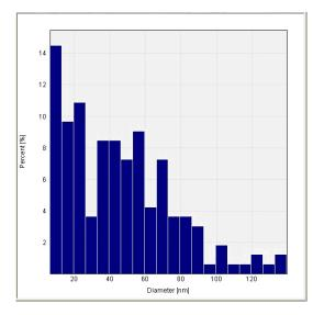
Fig. 2b. Grain size distribution histogram, sample no.2
