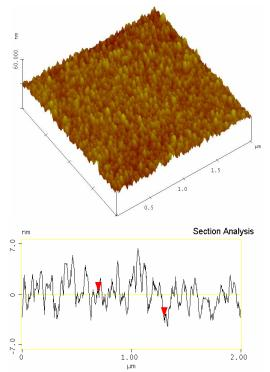
Fig. 1a. TM-AFM images showing 3D surface topography, 2x2 µm<sup>2</sup> and section analysis, sample no. 1
