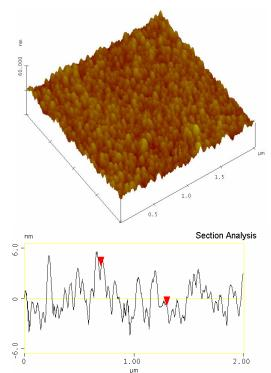
Fig. 1b. TM-AFM images showing 3D surface topography,  $2x2 \ \mu m^2$  and section analysis, sample no. 2.
