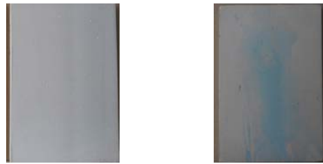
Acrylic coating with ZnO/SBA-15 composite after 30 days exposure to sunlight Acrylic coating without ZnO/SBA-15 composite after 30 days exposure to sunlight
