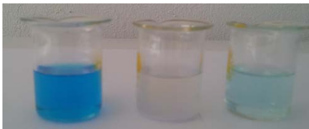
a) 1 % methylene blue aqueous solution unexposed to the sun light b) 1 % methylene blue aqueous solution and 0.1 g composite exposed to the sun light c) 1 % methylene blue aqueous solution exposed to the sun light
