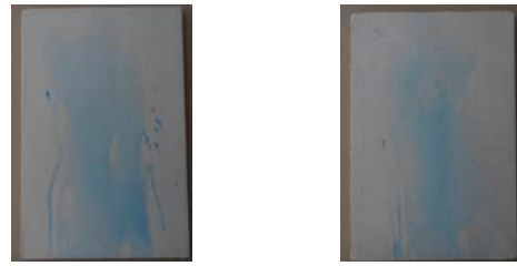
Acrylic coating with ZnO/SBA-15 composite before exposure Acrylic coating without ZnO/SBA-15 composite before exposure
