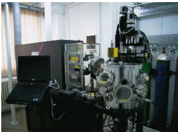
Fig. 1. PLD 2000 Workstation (PVD Products Ltd.), using 193 nm and 248 nm lasers (color online)
