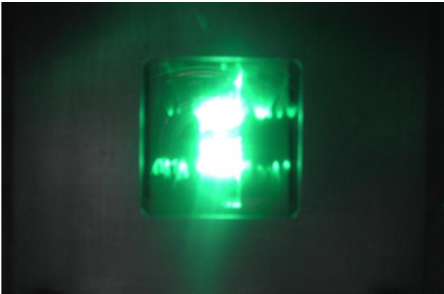
Fig. 7. Light emission from LAMIC thin silicon film annealed at 190+100 \text{ mJ/cm}^2 tested using an ITO coated phosphor anode plate in vacuum (color online)
