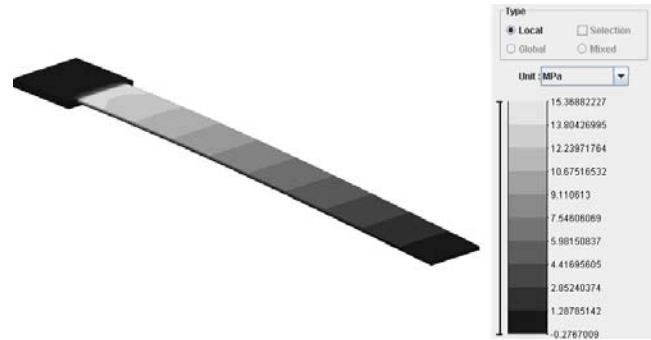
Fig.9. Finite element analysis of the bending stress of a microcantilever 200 \times 30 \times 1.9 \mu\text{m} .
