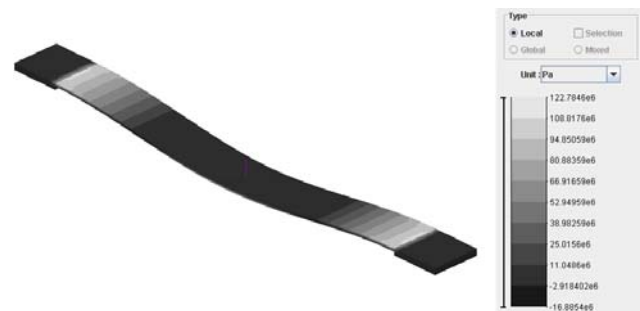
Fig.10. Finite element analysis of the bending stress of a microbridge 200 \times 30 \times 1.9 \mu\text{m} .
