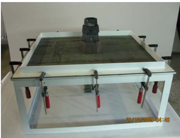
Fig. 1. Flexural load-unload test detail. Sandwich panel clamped on contour.
