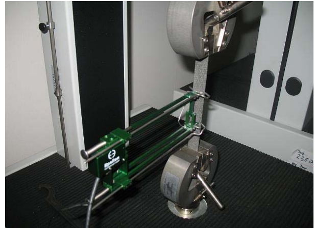
Fig. 2. Three-point bend load-unload test detail. Sandwich panel supported linearly on two opposite edges.
