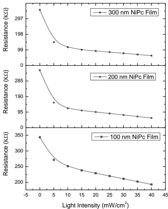
Fig. 4. AC resistance-irradiance relationships for OPTs based on nickel phthalocyanine with NiPc thickness of 100 nm, 200 nm and 300 nm
