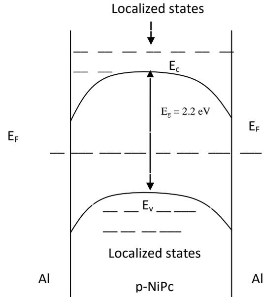
Fig. 7. An energy-band diagram of nickel phthalocyanine based transistor with two Al/p-NiPc metal-semiconductor Schottky junctions
