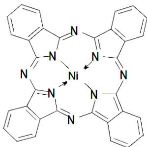
Fig. 1. Molecular structure of the nickel phthalocyanine used as a p-type organic semiconductor
