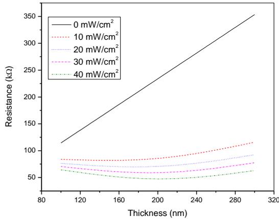
Fig. 6. AC resistance-thickness responses for the nickel phthalocyanine based OPTs at different irradiances
