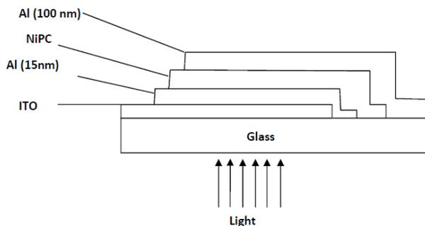
Fig. 3. Cross-sectional view of the fabricated organic transistor
