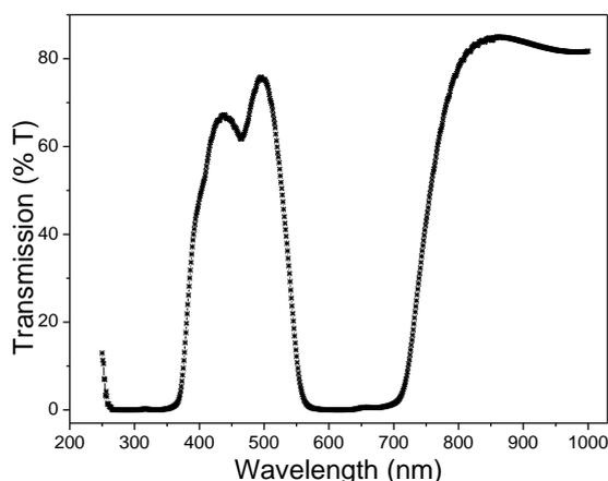
Fig. 2. UV-VIS transmission spectrum of the nickel phthalocyanine thin film (300 nm thickness)
