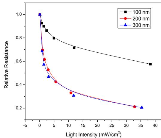
Fig. 5. Relative resistance-irradiance relationships for the nickel phthalocyanine based OPTs where NiPc thickness was 100 nm, 200 nm and 300 nm
