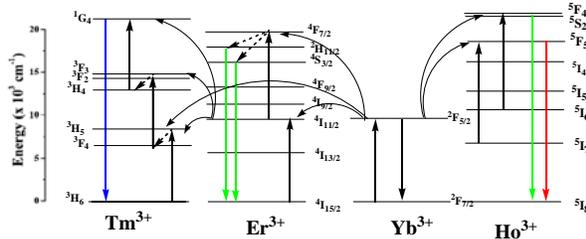
Fig. 6. Energy level diagram of the  $\text{Tm}^{3+}$ ,  $\text{Er}^{3+}$ ,  $\text{Yb}^{3+}$ , and  $\text{Ho}^{3+}$  ions as well as the proposed upconversion mechanism to produce the blue, green, orange, and white emission for the  $\text{Yb}^{3+}/\text{Tm}^{3+}/\text{Er}^{3+}/\text{Ho}^{3+}$ -doped  $\text{Na}_{0.5}\text{Gd}_{0.5}\text{WO}_4$  nanocrystals upon 980 nm semiconductor laser excitation.
