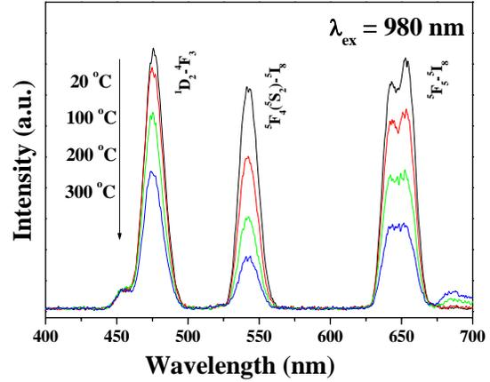
Fig. 7. Temperature dependence of UC luminescence spectra of  $\text{Na}_{0.5}\text{Gd}_{0.5}\text{WO}_4:10\%\text{Yb}^{3+}, 1\%\text{Tm}^{3+}, 0.4\%\text{Ho}^{3+}$  nanocrystals upon 980 nm semiconductor laser excitation.
