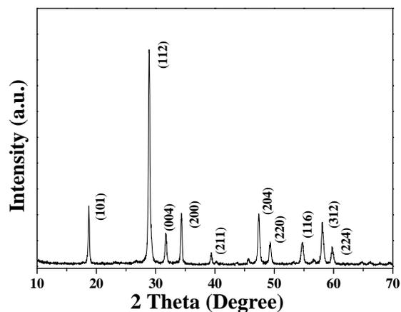
Fig. 1. XRD pattern of as-prepared  $\text{Na}_{0.5}\text{Gd}_{0.5}\text{WO}_4:10\%\text{Yb}^{3+}, 1\%\text{Tm}^{3+}, 0.4\%\text{Ho}^{3+}$  nanocrystals.
