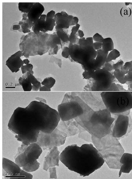
Fig. 2. TEM images of as-prepared  $\text{Na}_{0.5}\text{Gd}_{0.5}\text{WO}_4:10\%\text{Yb}^{3+}, 1\%\text{Tm}^{3+}, 0.4\%\text{Ho}^{3+}$  nanocrystals, (a)  $0.2 \mu\text{m}$  scale, (b)  $200 \text{ nm}$  scale.
