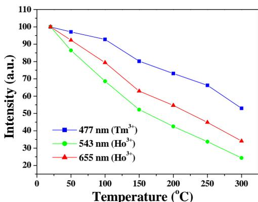
Fig. 8. Relative emission intensities of the blue, green, and red UC luminescence of Na<sub>0.5</sub>Gd<sub>0.5</sub>WO<sub>4</sub>:10%Yb<sup>3+</sup>,1%Tm<sup>3+</sup>, 0.4%Ho<sup>3+</sup> nanocrystals as a function of temperature.
