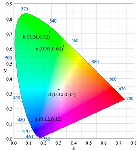
Fig. 4. CIE (X, Y) coordinate diagram (CIE-1931) showing the chromaticity points of the emissions in the Na<sub>0.5</sub>Gd<sub>0.5</sub>WO<sub>4</sub> doped with 10%Yb<sup>3+</sup>/1%Tm<sup>3+</sup> (a), 10%Yb<sup>3+</sup>/1%Er<sup>3+</sup> (b), 10%Yb<sup>3+</sup>/1%Ho<sup>3+</sup> (c), and 10%Yb<sup>3+</sup>/1%Tm<sup>3+</sup>/0.4%Ho<sup>3+</sup> (d) under 980 nm semiconductor laser excitation.
