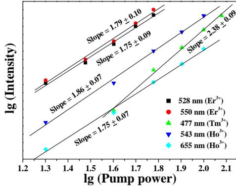
Fig. 5. Pump power dependence of the blue, green, and orange UC luminescence in  $\text{Na}_{0.5}\text{Gd}_{0.5}\text{WO}_4$  nanocrystals doped with  $\text{Tm}^{3+}$ ,  $\text{Er}^{3+}$  and  $\text{Ho}^{3+}$ .
