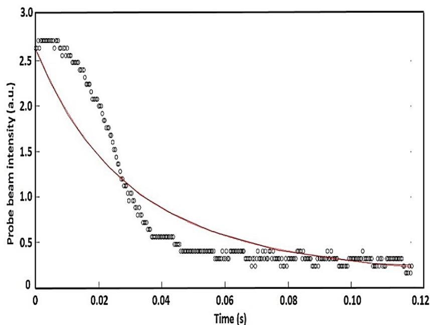
Fig. 5. Thermal lensing curve of Ag-CuNPs@PVA (color online)
