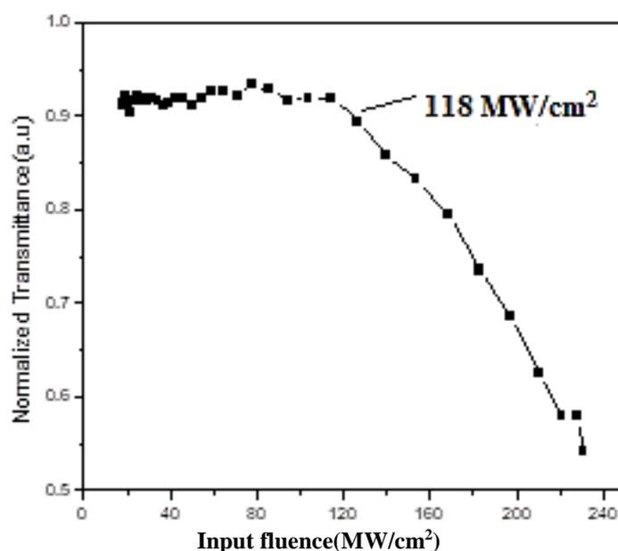
Fig. 4. Optical limiting curve of Ag-CuNPs@PVA
