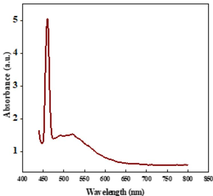
Fig. 1. Absorption spectrum of Ag-CuNPs@PVA (color online)
