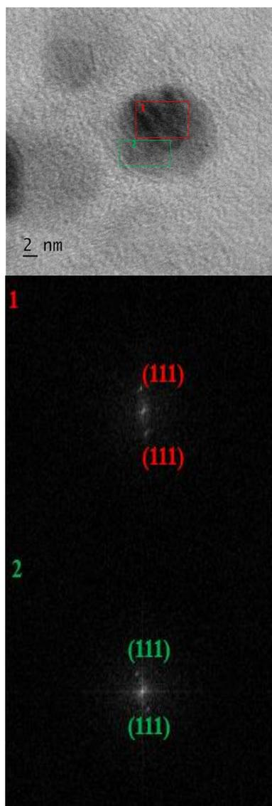
Fig. 2. TEM image of Ag-CuNPs@PVA (Fig 2 above). FFT pattern of CuNPs (Fig 1 below) and AgNPs (color online)
