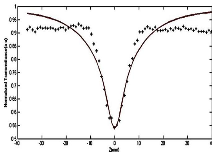
Fig. 3. Open-aperture Z-scan curve of Ag-CuNPs@PVA
