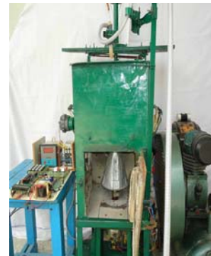
Fig. 4. Photograph of the microcontroller circuit & inclined substrate for spray pyrolysis set up.
