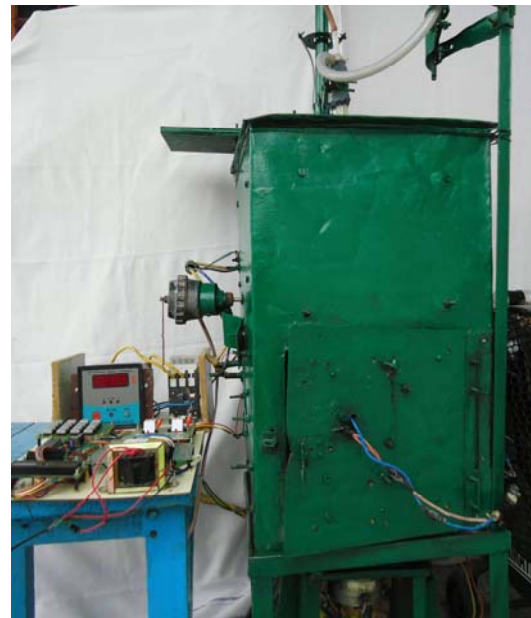
Fig. 4. Photograph of the microcontroller circuit with spray pyrolysis set up.
