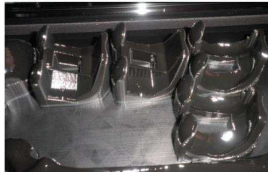
Fig. 16. Printing process of the knee implants by PJP technology.
