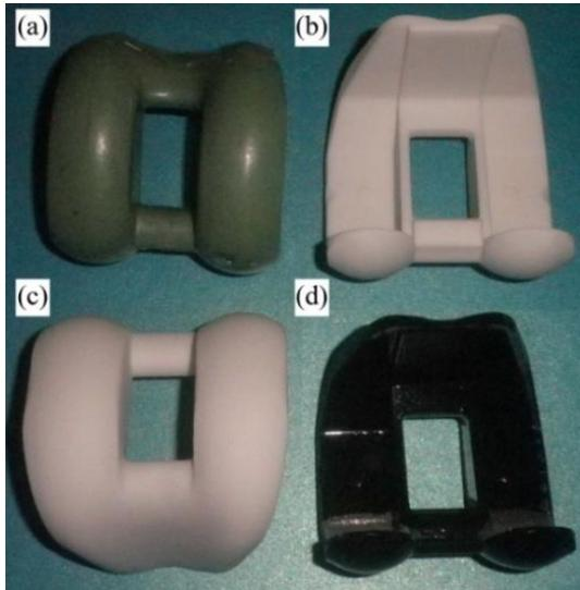
Fig. 20. Finished knee implant pattern models:(a) wax pattern, (b) SLS model, (c) 3DP model and (d) PJP model.
