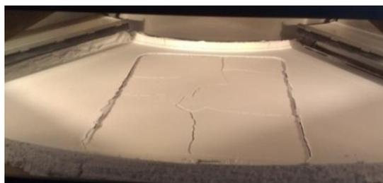
Fig. 8. SLS printing process of the knee implants.
