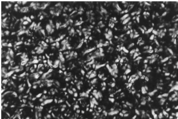
Fig. 3 Electro-hydrodynamics at a 7 V d.c. voltage, destroying the cross-like domains and  $\pi$ -walls viewed under a polarizing microscope in crossed nicols. The (+) pole is on the upper electrode,  $T = 142$  °C. The long side of the photograph measures 790  $\mu\text{m}$ .
