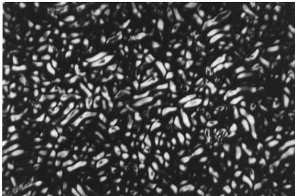
Fig. 2. Cross-like domains and  $\pi$ -walls above the threshold ( $U = 2.5$  V) viewed under a polarizing microscope in crossed nicols. The applied d.c. voltage is 5 V, the (+) pole is on the upper electrode surface coinciding with the microphotograph focal plane,  $T = 142$  °C. The long side of the photograph measures 790  $\mu\text{m}$ .
