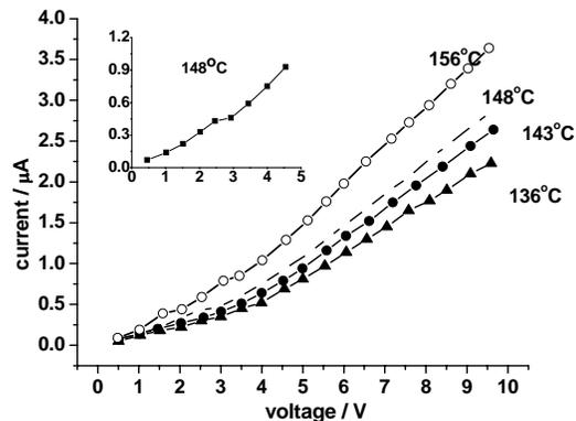
Fig. 4. Current-voltage characteristics of the nematic layer at: 136°C, 143°C, 148°C. The upper curve is drawn at 156°C, in the isotropic phase.
