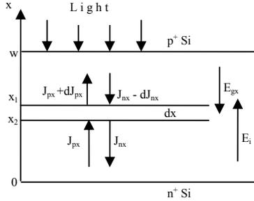
Fig. 1. Scheme of cross section of a solar cell under illumination (p+-side).
