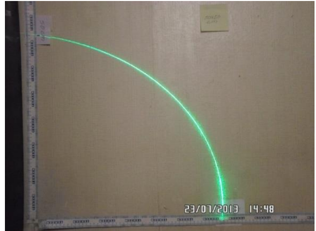
Fig. 1. Laser is bent towards the left as a quarter circle (color online)
