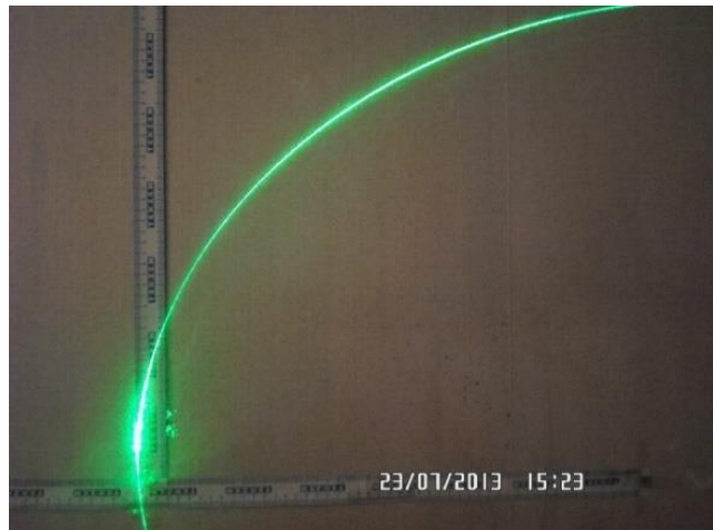
Fig. 2. Laser is bent towards the right as parabolic (color online)
