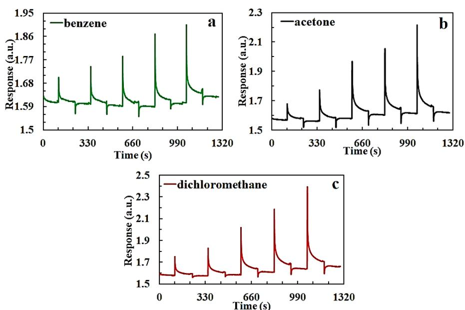
Fig. 10. The photodetector response of NHDACx optical LB thin film with 7.9 nm thickness for a) benzene b) acetone c) dichloromethane vapors at different concentrations (color online)
