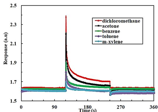
Fig. 12. The photodetector response of NHDACx optical LB thin film with 7.9 nm thickness for different five vapors (color online)
