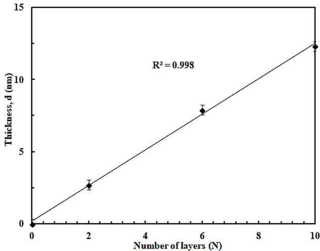
Fig. 8. Modeled layer thickness as a function of layer number for NHDACx LB layers.
