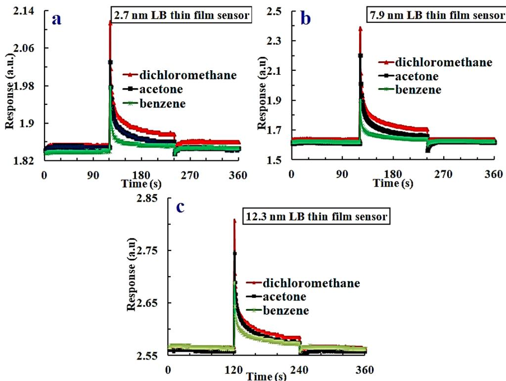
Fig. 9. The photodetector response of NHDACx LB film with a) 2.7 nm thickness b) 7.9 nm thickness c) 12.3 nm thickness against organic vapors (color online)
