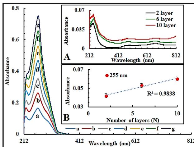
Fig. 6. UV-Vis spectra of the NHDACx in chloroform solution at different concentrations. Inset: A the NHDACx LB film on quartz glass substrate B linear increase of absorbance as a function of layer number (color online)
