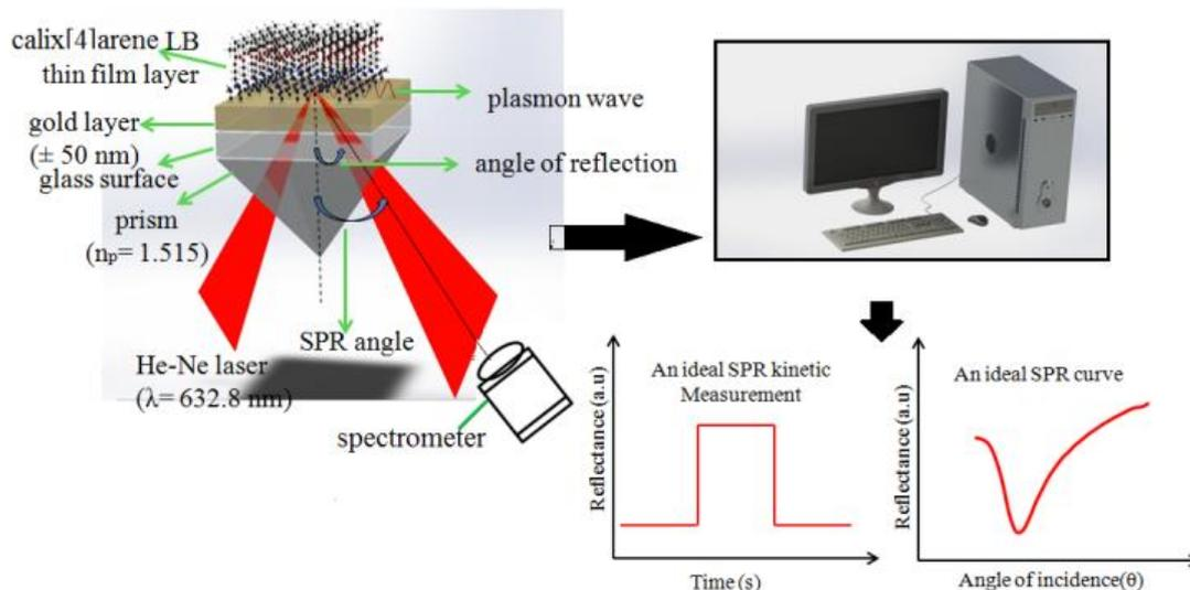
Fig. 2. A schematic diagram of the surface plasmon resonance measurement system (color online)
