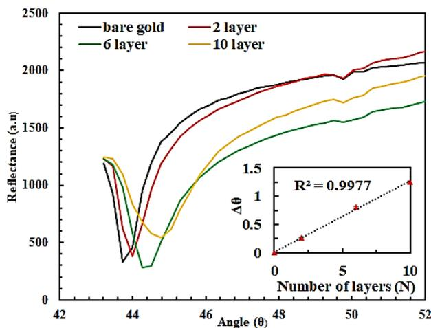
Fig. 5. SPR curves of NHDACx LB films with increase in thickness. Inset: Linear increase of thickness as a function of number of bilayers (color online)
