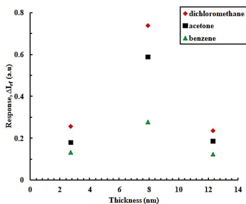
Fig. 11. Response-thickness diagram for NHDACx based optical sensor under exposure of dichloromethane, acetone, and benzene at saturated concentration (color online)
