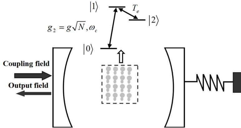
Fig. 1. Schematic of a hybrid optomechanical system with QDMs. Left (right) mirror is fixed (vibrating). The mechanical resonator couples the cavity field through the radiation pressure. The asymmetrical QDM system [50] with different band structure couples the cavity field with the collective strength  $g_2$ . Interdot tunneling in the QDMs can be controlled by applying a gate electrode between them[58,59]
