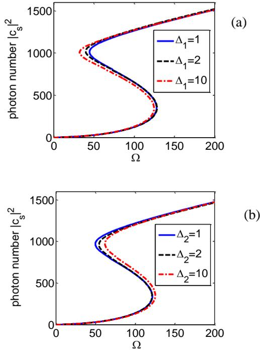
Fig. 7. Photon number  $|c_s|^2$  of the optomechanical cavity vs. the frequency detuning (a)  $\Delta_1 = 1, 2, 10$  with  $\Delta_2 = 0$ , and (b)  $\Delta_2 = 1, 2, 10$  with  $\Delta_1 = 0$ . The other parameters are  $T_e = 1, \gamma_1 = \gamma_2 = 1, \kappa = 1, \Delta_c = -10, g_1 = 0.1, g_2 = 1$  (color online)
