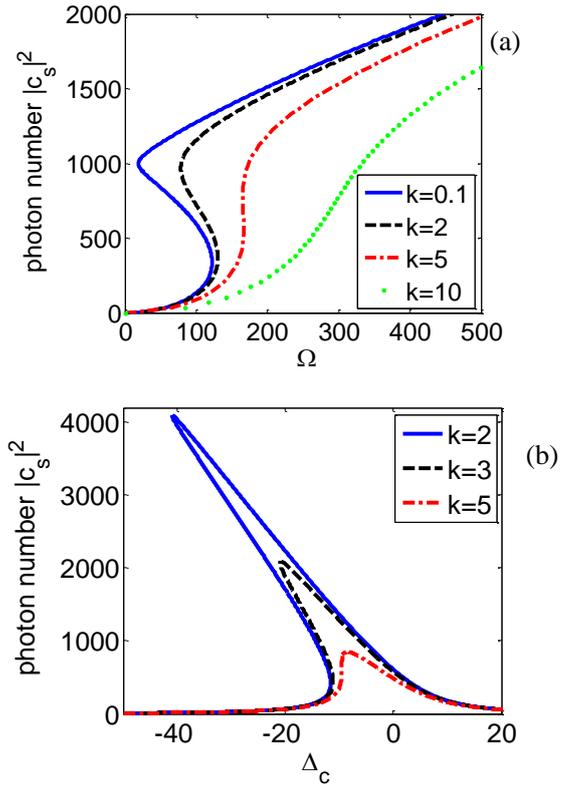
Fig. 4 (a) Photon number  $|c_s|^2$  of the optomechanical cavity vs. the Rabi frequency  $\Omega$  of the coupling laser for different decay rate  $K=0.1, 2, 5$  and  $10$  with  $\Delta_c = -10$ .
