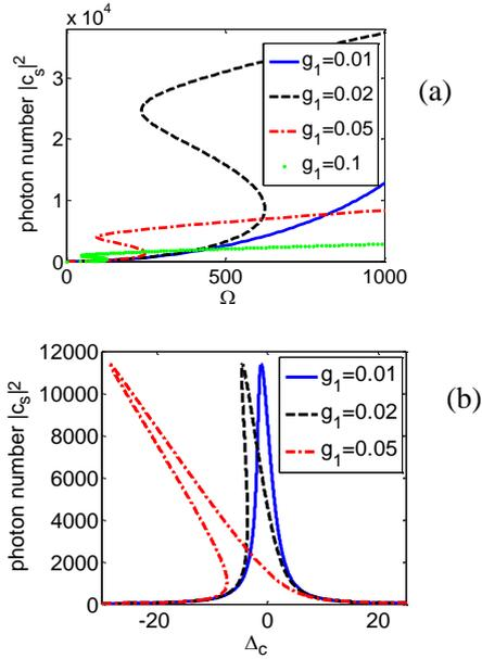
Fig. 5 (a) Photon number  $|c_s|^2$  of the optomechanical cavity vs. the coupling strength  $g_1 = 0.01, 0.02, 0.05$  and  $0.1$  with  $\Delta_c = -10$ . (b) Photon number  $|c_s|^2$  of the optomechanical cavity vs. frequency detuning  $\Delta_c$  for different coupling strength  $g_1 = 0.01, 0.02, 0.05$  with  $\Omega = 160$ . The other parameters are  $T_e = 1, \gamma_1 = \gamma_2 = 1, \Delta_1 = \Delta_2 = 0, g_2 = 1$  (color online)
