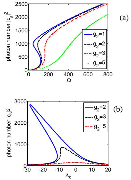
Fig. 6. (a) Photon number  $|c_s|^2$  of the optomechanical cavity vs. the coupling strength  $g_2 = 1, 2, 3$  and  $5$  with  $\Delta_c = -10$ . (b) Photon number  $|c_s|^2$  of the optomechanical cavity vs. frequency detuning  $\Delta_c$  for different coupling strength  $g_2 = 2, 3$  and  $5$  with  $\Omega = 160$ . The other parameters are  $T_e = 1, \gamma_1 = \gamma_2 = 1, \Delta_1 = \Delta_2 = 0, g_1 = 0.1$  (color online)
