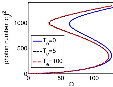
Fig. 3 Photon number  $|c_s|^2$  of the optomechanical cavity vs. the Rabi frequency  $\Omega$  of the coupling laser for different tunneling strength  $T_e=0, 5$  and  $100$ . The other parameters are  $\kappa = 1, \gamma_1 = \gamma_2 = 1,$
