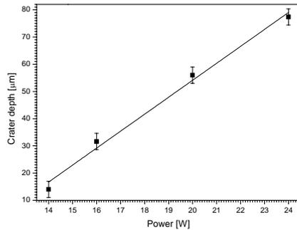
Fig. 3. The ablation crater depth at different laser beam power. The distance for which the temperature is above 100 °C.
