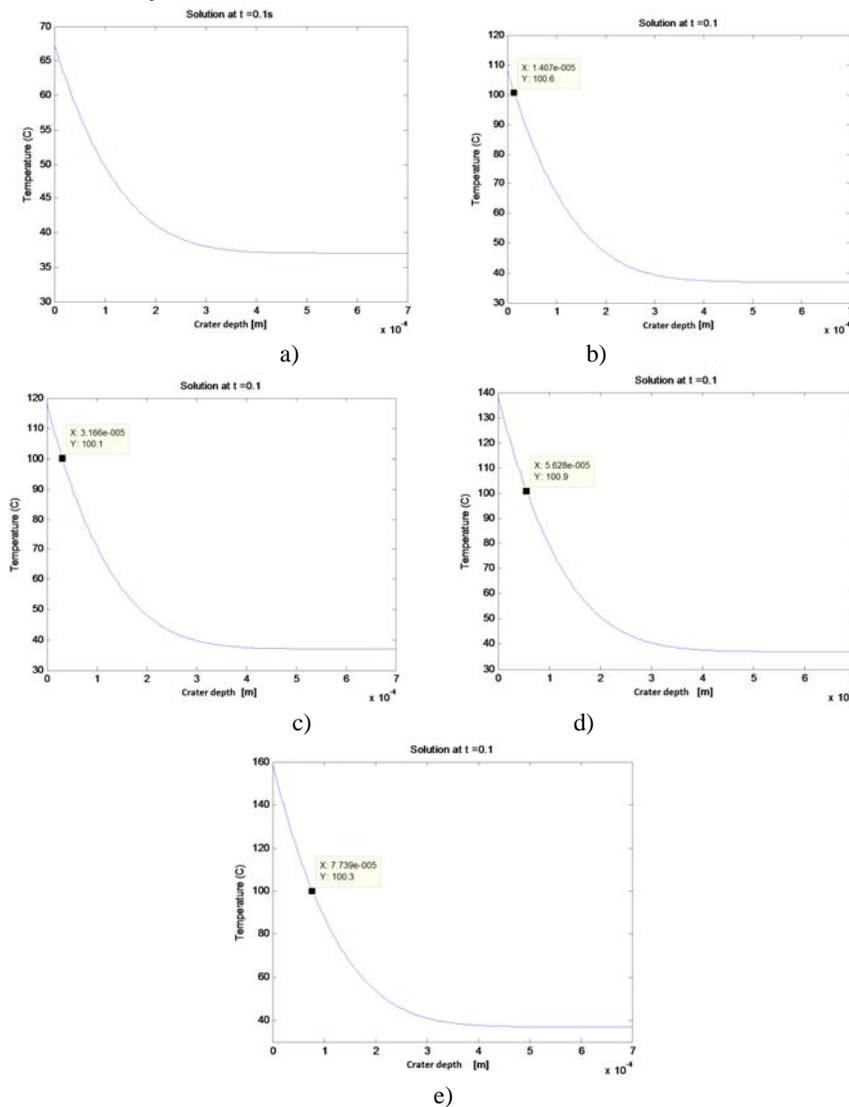
Fig. 2. Temperature distribution in the crater ablation depth and the maximum temperature at  $t=0.1$  sec: a)  $P=6$  W, b)  $P=14$  W, c)  $P=16$  W, d)  $P=20$  W, e)  $P=24$  W
