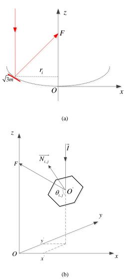
Fig. 3. (a) The side-view of hexagon-facet concentrator (b) The position of hexagonal facet (row=i; columns = j)
