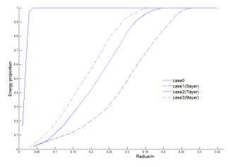
Fig. 6. The energy distribution radially of different solar concentrator
