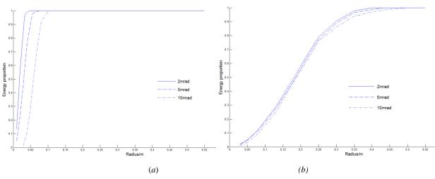
Fig. 7. (a) The energy distribution radially of paraboloid concentrator with different composition error (b) The energy distribution radially of new kind concentrator with different composition error
