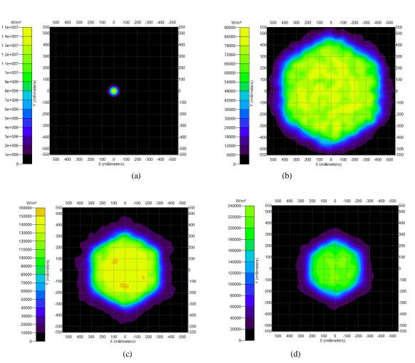
Fig. 5. Uniformity of the receiver:(a) paraboloid (b)5-layer (c)7-layer (d)9-layer
