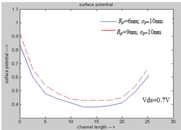
Fig. 4. Surface Potential variation along the channel length.
