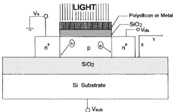
Fig. 2 Schematic diagram of SOI MOSFET under illumination.
