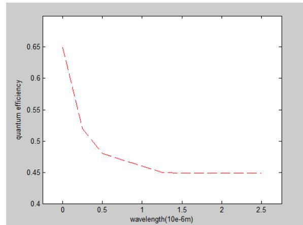
Fig. 10. Variation of quantum efficiency with operating wavelength.
