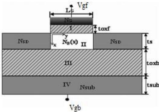
Fig.1. Cross section of fully depleted SOI MOSFET.
