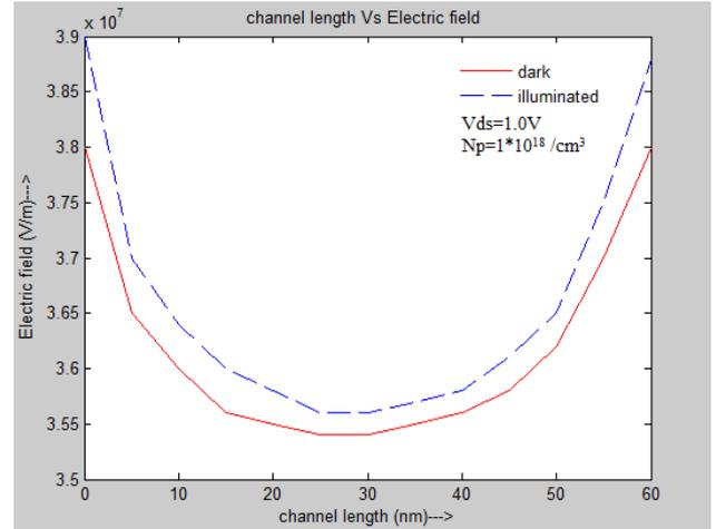
Fig. 5. Variation of Electric field under dark and illuminated conditions.
