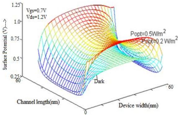
Fig. 3. Variation of surface potential for non-uniformly doped channel.
