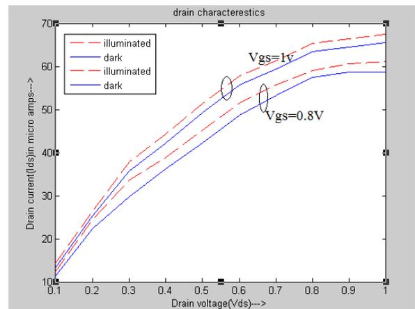
Fig. 6. Variation of Drain current under dark and illuminated conditions.
