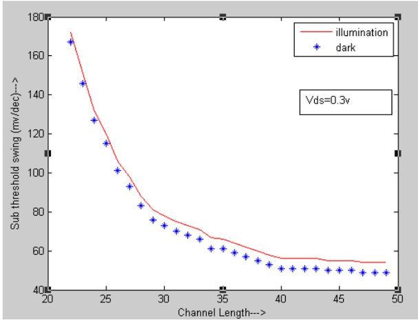
Fig. 7. Sub Threshold Swing along the length of the channel under dark and illuminated conditions.
