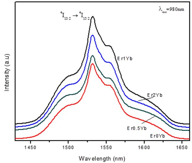
Fig. 3. Near Infrared emission spectra of the Er-Yb codoped boro-tellurite glasses
