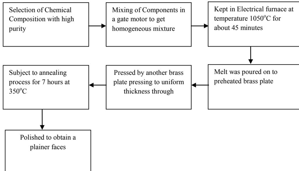
Fig. 1. Block diagram showing the procedure for preparation of the proposed glass
