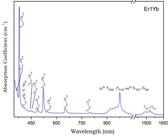
Fig. 2. Absorption spectrum of the Er-Yb co-doped Er1Yb glass in the UV-Vis-NIR region
