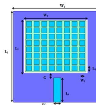
Fig. 1. Meshed patch antenna 7x7 array structure
