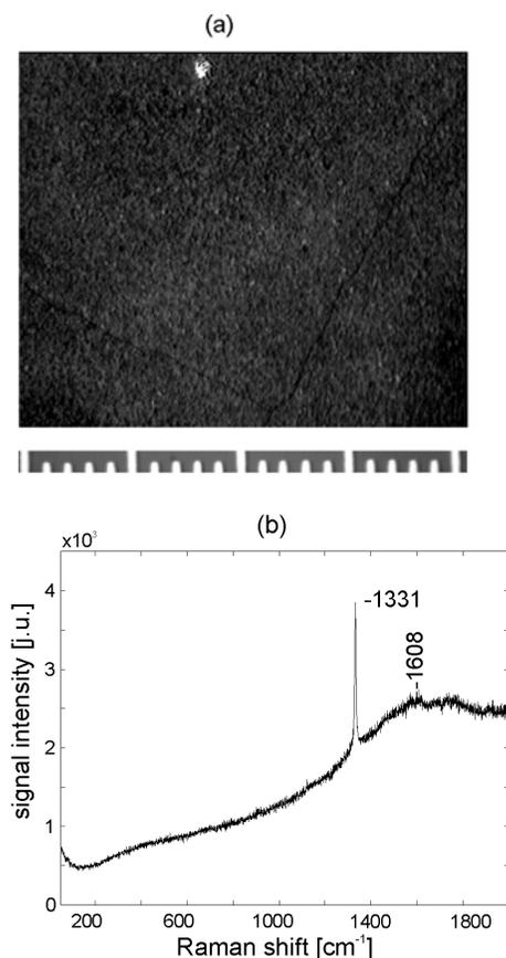
Fig. 6. Microscopic image (a) and micro-Raman spectrum (b) of microwave-plasma-CVD polycrystalline diamond film; length unit equal to 10 μm.
