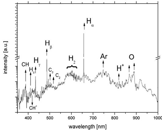
Fig. 4. Typical emission spectra of the H<sub>2</sub>:CH<sub>4</sub> plasma (microwave power 800 W and gas flow 25 sccm).
