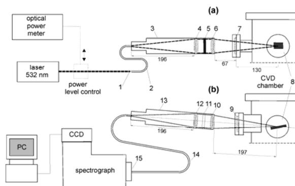
Fig. 3. Design of Raman system for monitoring of  $\mu\text{PA}$  CVD process: (a) excitation part, (b) acquisition part; 1 - coupler, 2 - optical fibre, 3 - excitation probe, 4, 6, 10, 12 - lenses, 5 - bandpass filter, 7, 9 - windows, 8 - growing film, 11 - notch filter, 13 - collecting probe, 14 - fibre bundle, 15 - adapter; dimensions are given in millimeters.
