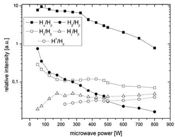
Fig. 5. Ratio of optical emission intensities of lines vs. microwave power.
