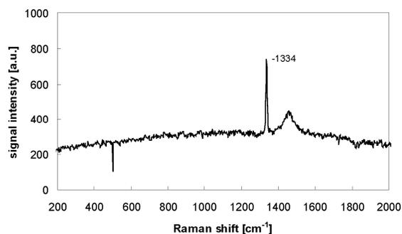
Fig. 7. Test spectrum of monocrystalline diamond recorded by the prototype of the dedicated Raman system for *in-situ* monitoring.
