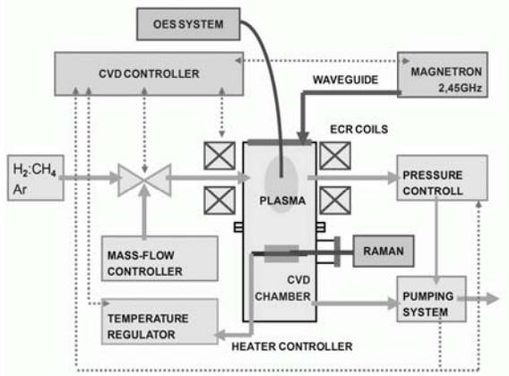
Fig. 1. Schematic diagram of experimental CVD system.
