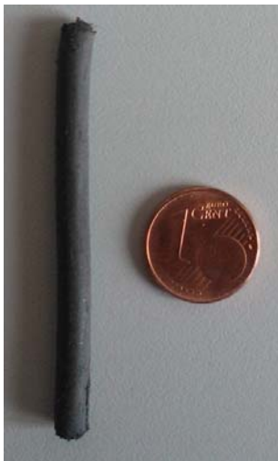
Fig. 3. Cylindrical sample of MAE for the torsion test.
