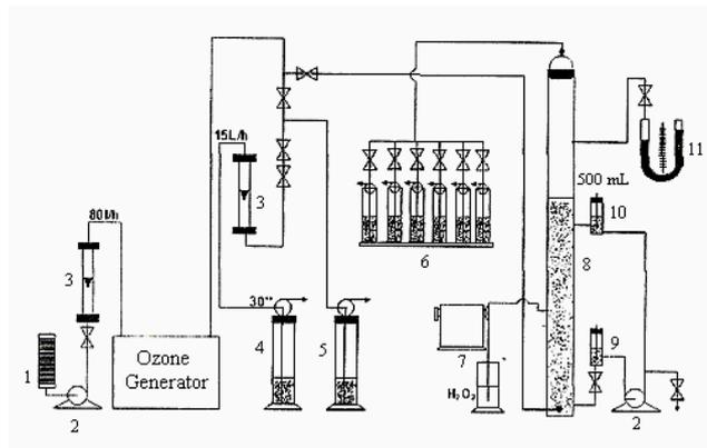
Fig. 2. Schematic representation of the ozonation system. 1 - Air dryer, 2 - recirculation pump, 3 - rotameters, 4 - ozone absorption vessel (for dosage), 5 - ozone absorption vessel (for the excess of ozone); 6 - battery residual ozone absorption vessels, 7 - peristaltic pump, 8 - oxidation column, 9 - pH meter, 10 - conductometer, 11 - manometer.
