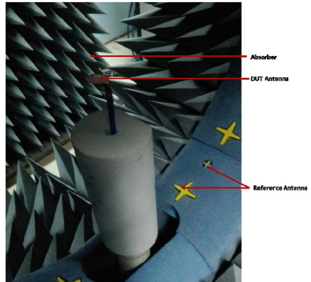
Fig. 5. Farfield characteristics measurement setup (Satimo nearfield measurement system)
