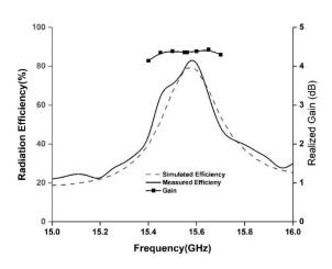
Fig. 8. Radiation efficiency and realized gain of the presented antenna
