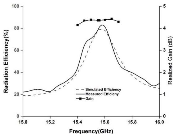
Fig. 8. Radiation efficiency and realized gain of the presented antenna
