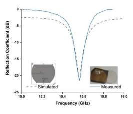
Fig. 3. Reflection coefficient of the presented antenna
