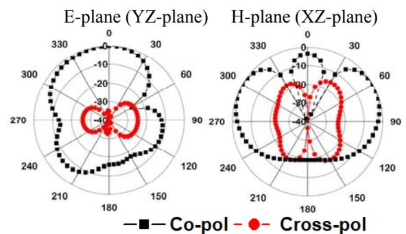
Fig. 6. Polar radiation pattern of the presented antenna at 15.56 GHz
