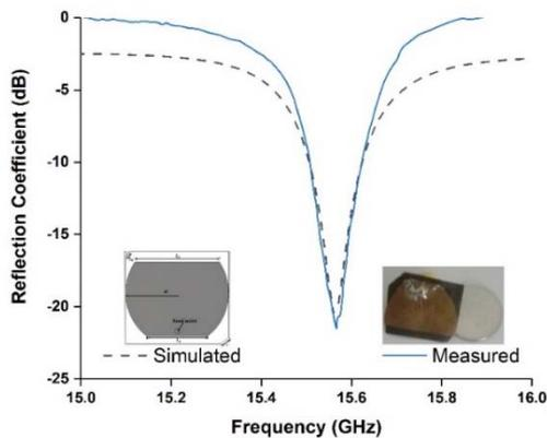
Fig. 3. Reflection coefficient of the presented antenna
