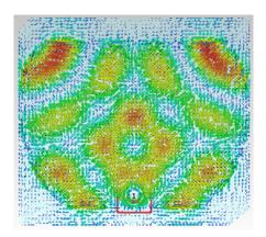
Fig. 4. Surface current distribution of the developed antenna at 15.56 GHz
