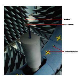
Fig. 5. Farfield characteristics measurement setup (Satimo nearfield measurement system)
