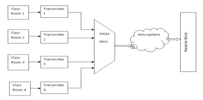
Fig. 1. Block Diagram of WDM Transceiver
