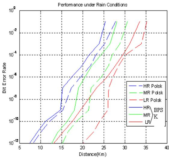
Fig. 5. BER Vs distance under rain conditions
