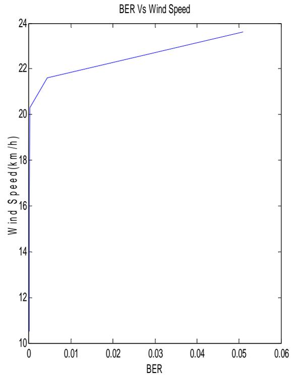
Fig. 10. BER Vs wind speed for 12 months (tricky weather conditions)
