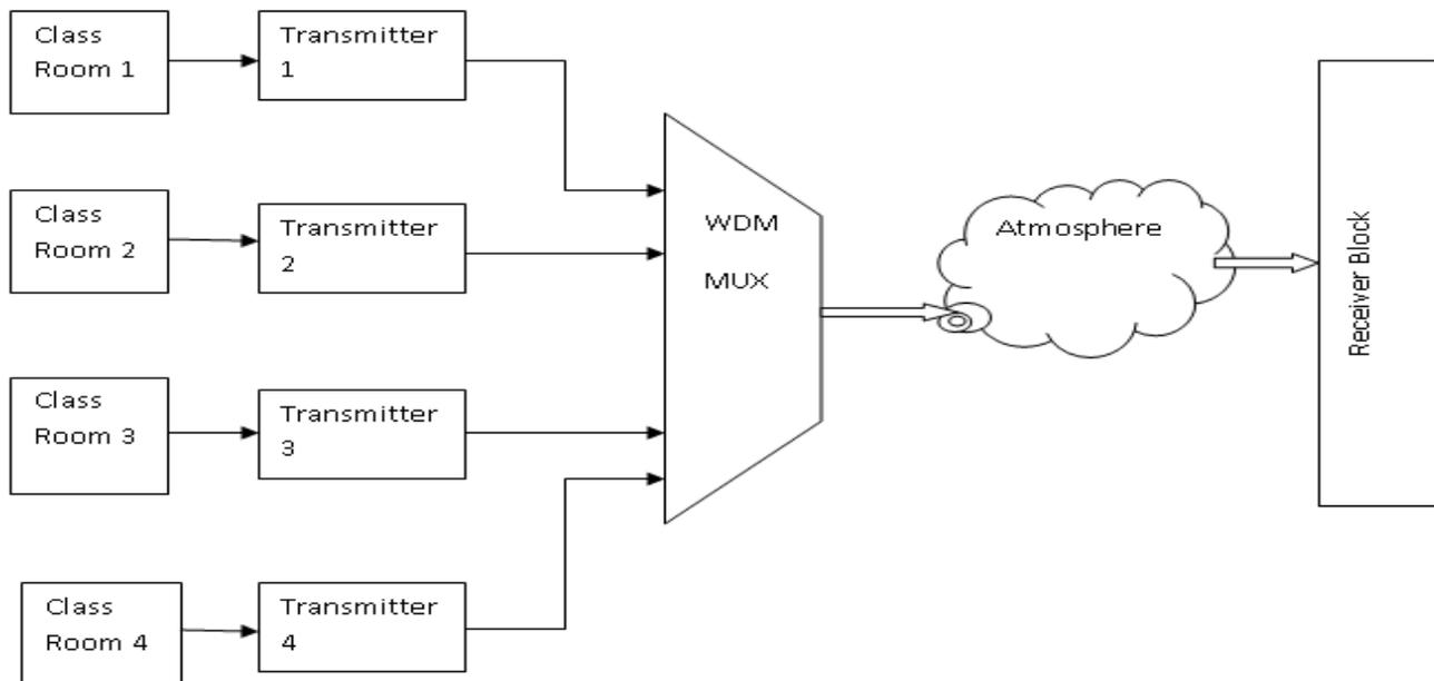
Fig. 1. Block Diagram of WDM Transceiver
