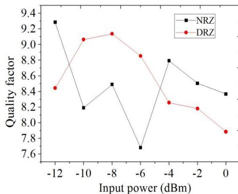
Fig. 3. The variation of the quality factor on input power without dispersion compensation technique
