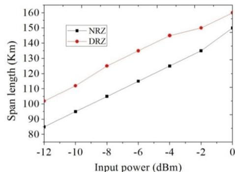
Fig. 6. The variation of the span length of the network on input power using FBG as dispersion compensation technique.
