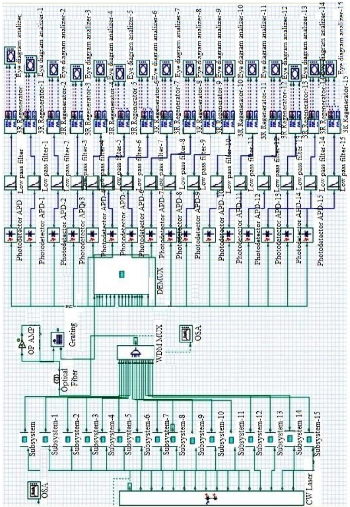
Fig. 2. Circuit diagram of the designed UDWDM PON.
