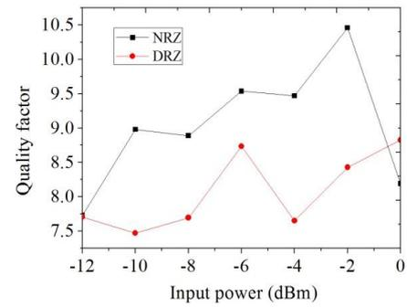
Fig. 4. The variation of the quality factor on input power using FBG as dispersion compensation technique
