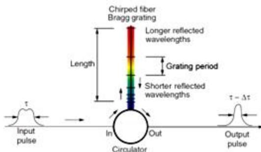
Fig. 1. Schematic of chirped FBG based dispersion compensation
