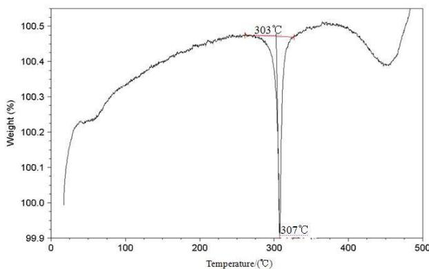
Fig.7 DTG curve of 3DAP for Nd<sub>83</sub>Fe<sub>77.1</sub>B<sub>6.4</sub>Co<sub>4</sub>Zr<sub>3</sub>Nb<sub>0.5</sub>V<sub>0.5</sub> alloy
