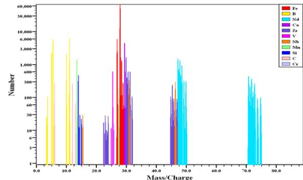
Fig.4 Mass spectrum of 3DAP for Nd<sub>8.5</sub>Fe<sub>77.1</sub>B<sub>6.4</sub>Co<sub>4</sub>Zr<sub>3</sub>Nb<sub>0.5</sub>V<sub>0.5</sub> alloy
