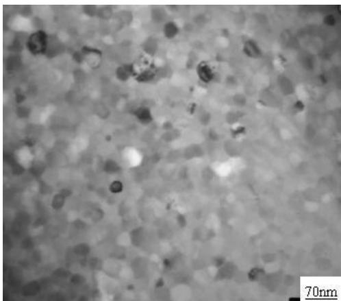
Fig.2 TEM micrographs of Nd<sub>8.5</sub>Fe<sub>77.1</sub>B<sub>6.4</sub>Co<sub>4</sub>Zr<sub>3</sub>Nb<sub>0.5</sub>V<sub>0.5</sub> ribbons annealed at 710 °C for 4 min
