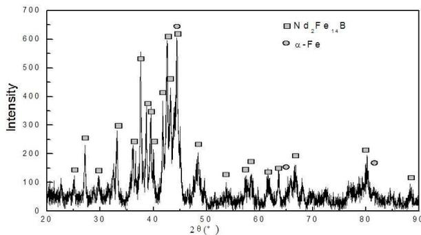
Fig.1 XRD spectrum of the Nd<sub>8.5</sub>Fe<sub>77.1</sub>B<sub>6.4</sub>Co<sub>4</sub>Zr<sub>3</sub>Nb<sub>0.5</sub>V<sub>0.5</sub> ribbons annealed at 710 °C for 4 min
