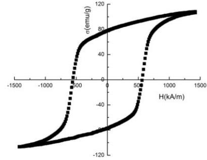
Fig.3 Hysteresis loops of Nd<sub>8.5</sub>Fe<sub>77.1</sub>B<sub>6.4</sub>Co<sub>4</sub>Zr<sub>3</sub>Nb<sub>0.5</sub>V<sub>0.5</sub> ribbons annealed at 710 °C for 4 min.
