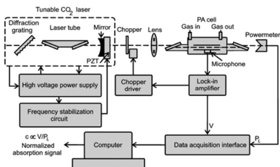
Fig. 2. Typical LPAS system for ethylene gas determination.
