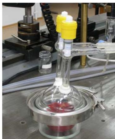
Fig. 3. The device used to contain fruits for the prelevation of the ethylene gas samples.
