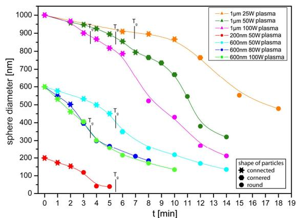
Fig. 3. Time dependence of the sphere diameter for 200, 600, and 1000 nm bead diameter NSL masks after air plasma treatment at different powers. The star-like symbols represent necked spheres, the hexagonal ones hexagonally distorted spheres and the filled circles rounded spheres.
