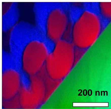
Fig. 4 Energy filtered cross-sectional TEM elemental maps of a 200 nm diameter PS double-layer mask on Si after 3 min air plasma treatment at 50 W. The sample was coated with 100 nm Co prior to specimen preparation. Colour code: Si=green, C=red, Co=blue.
