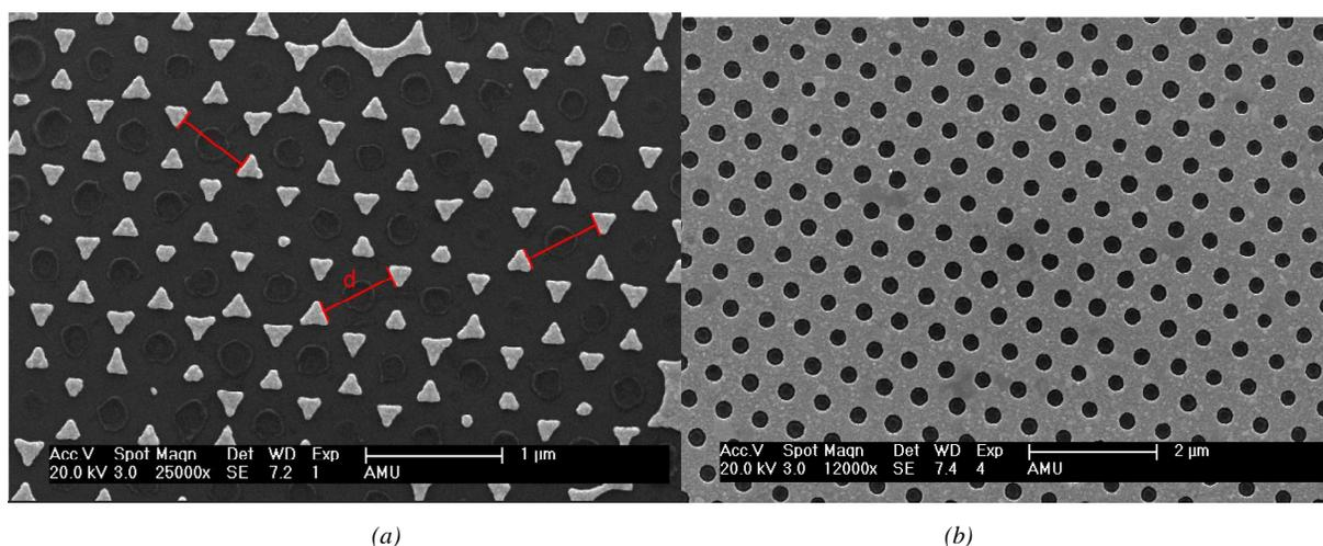
Fig. 1. Ag dot array obtained using an unmodified 600 nm diameter NSL mask (a) and a 600 nm diameter mask and plasma treatment for 4 min at 100 W (b). Both images exhibit the sample with the mask removed.
