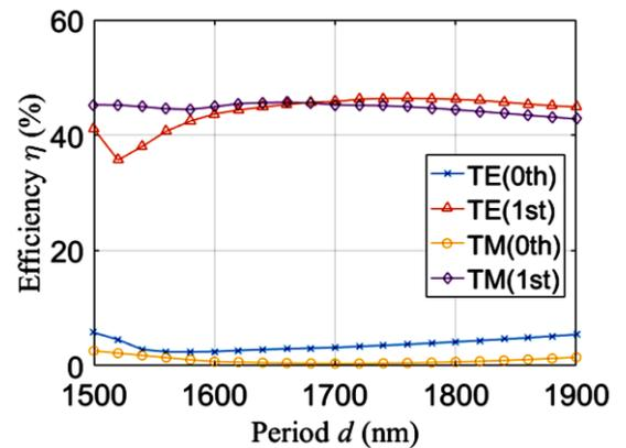
Fig. 4. (Color online) The diffraction efficiency corresponding to the period at wavelength of 800 nm with duty cycle of 0.28 under normal incidence (color online)
