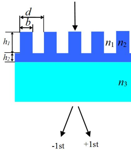
Fig. 1. (Color online) The schematic diagram of the grating with the zeroth order suppressed at wavelength of 800 nm with duty cycle of 0.28 under normal incidence (color online)
