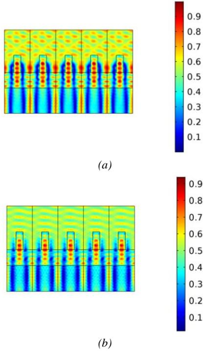
Fig. 3. (Color online) Normalized field magnitude distribution for the grating with the zeroth order suppressed under normal incidence: (a) TE polarization, (b) TM polarization (color online)
