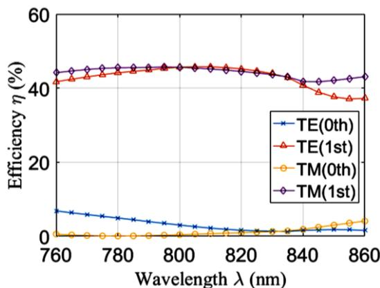
Fig. 6. (Color online) The efficiency corresponding to the incident wavelength with duty cycle of 0.28 under normal incidence (color online)
