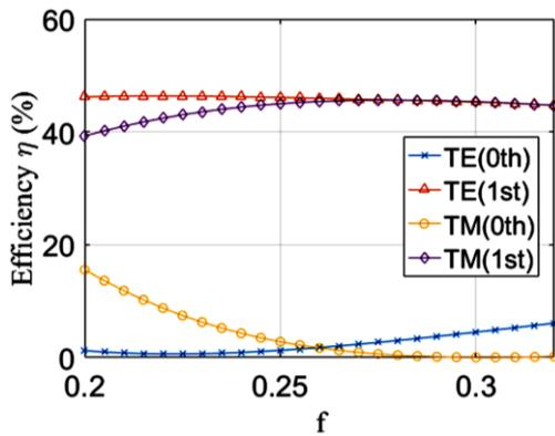
Fig. 5. (Color online) The diffraction efficiency corresponding to the duty cycle at wavelength of 800 nm under normal incidence (color online)
