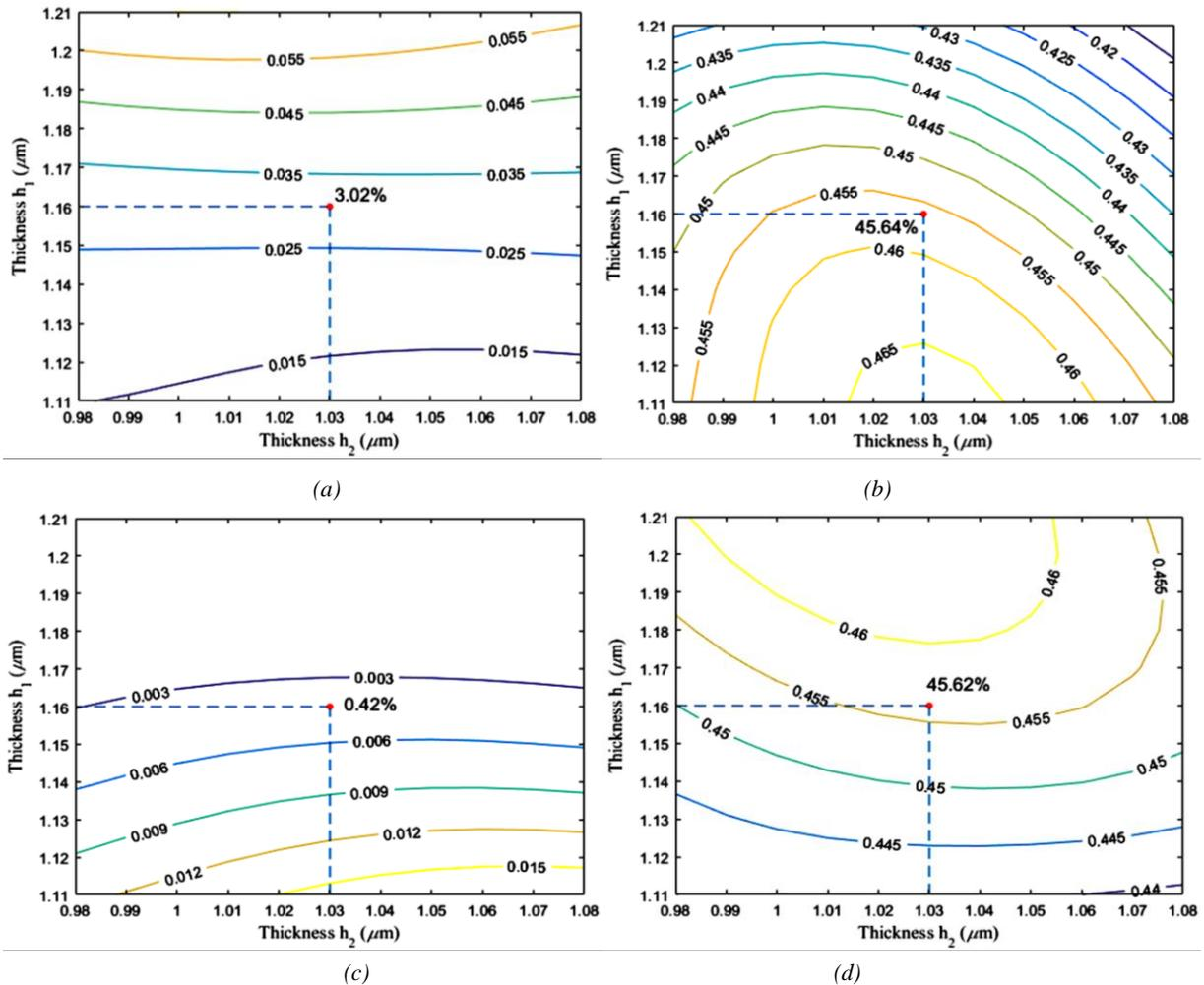
Fig. 2. Efficiencies in two orders for the grating versus the grating groove depth and the thickness of the connecting layer for both two polarizations at wavelength of 800 nm under normal incidence: (a) the 0th order for TE polarization, (b) the 1st order for TE polarization, (c) the 0th order for TM polarization, (d) the 1st order for TM polarization (color online)
