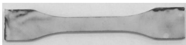
Fig. 5. PA6/carbon fiber laminate specimen for tensile test
