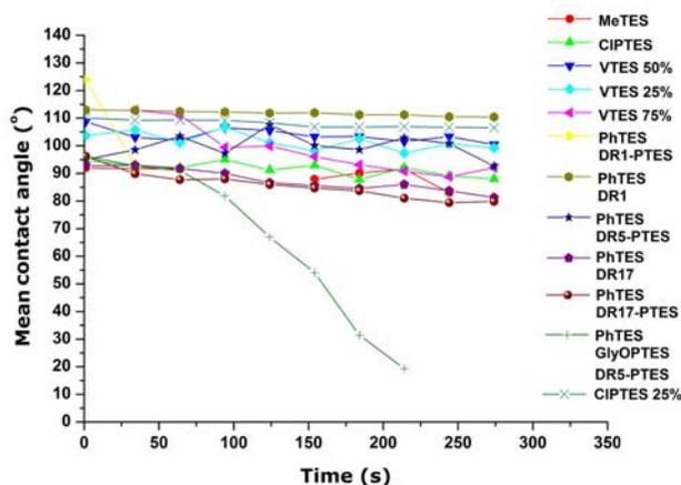
Fig. 4. The mean contact angle on PES fabrics coated with nanosols
