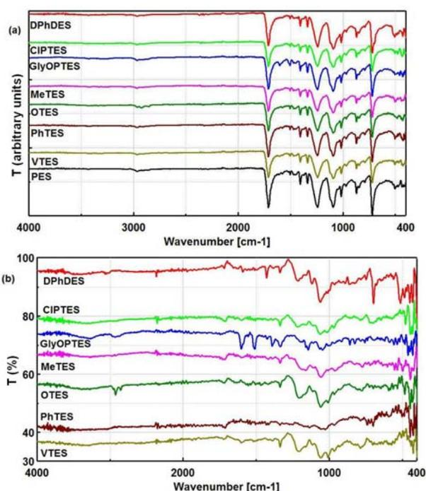
Fig.1. ATR-FTIR spectra of PES fabrics coated with nanosols (a) and of the coatings obtained by subtracting the PES spectrum (b)
