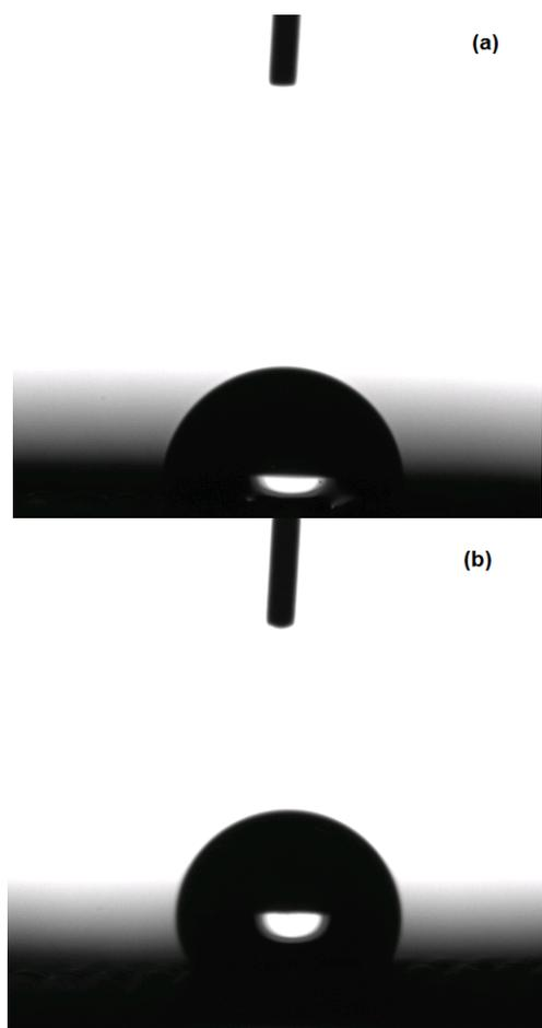
Fig. 5. Images of water drops on the surface of PES fibers coated with hybrids containing (a) PhTES/GlyOPTES=25/25 and (b) CIPTES
