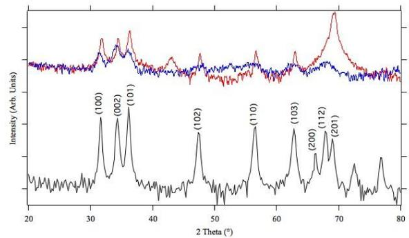
Fig. 3. XRD spectra of ZnO target (black) and thin films: 50fs pulse durations with 8mJ energy (red), 10ps pulse durations with 45mJ energy (blue).
