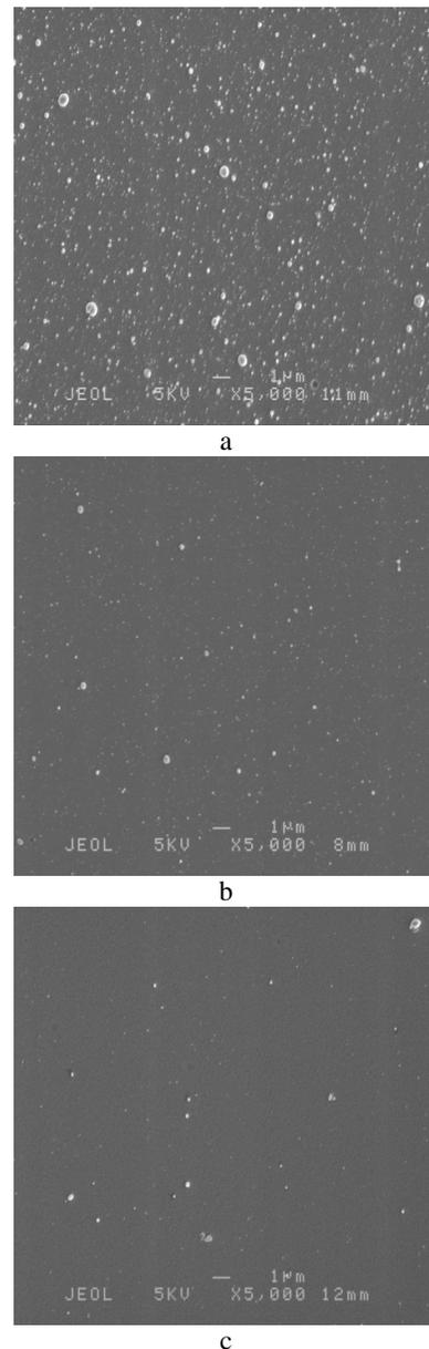
Fig. 5 - SEM images of the surfaces of films produced with 45mJ and pulse durations of (a) 200fs, (b) 10ps and (c) 275ps.
