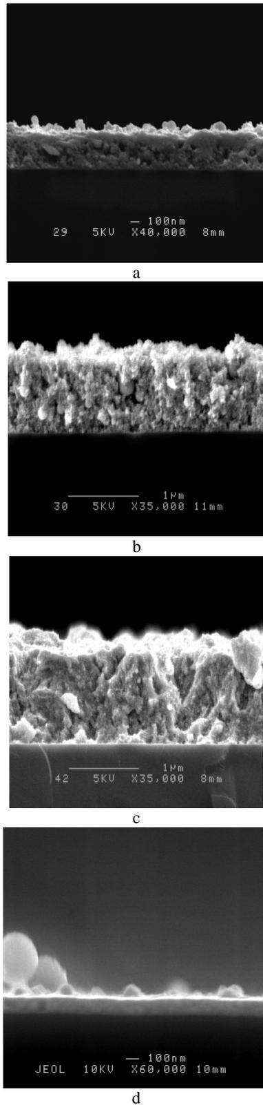
Fig. 4. Cross-section SEM images of films produced with 200fs pulses and energies of (a) 4.6mJ, (b) 8mJ, (c) 20mJ and (d) 45mJ.
