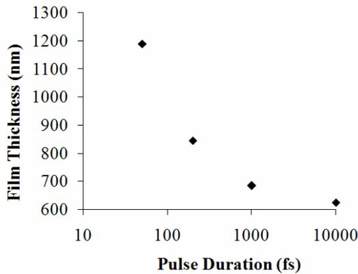
Fig. 1. Thickness of PLD grown ZnO films produced at a laser beam energy of 8mJ and measured on SEM cross-section images as a function of the laser pulse duration.
