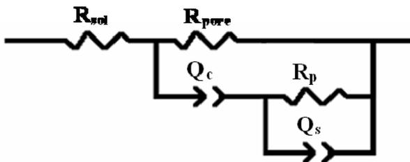
Fig. 3. Equivalent circuit for two-layer model: a compact inner layer and a porous outer layer, with unsealed pores
