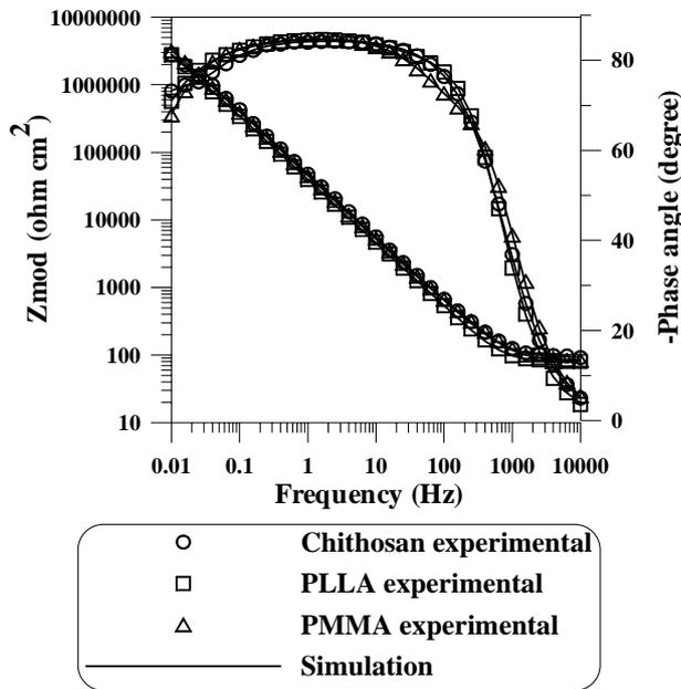
Fig. 2. Bode plot of the coated/NiTi samples in artificial saliva measured at open circuit potential.
