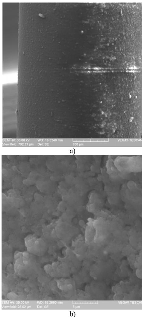
Fig. 1. SEM figures of a Nitinol wire covered with PMMA superficial layer a) 500 x and b) 10000 x power amplification.
