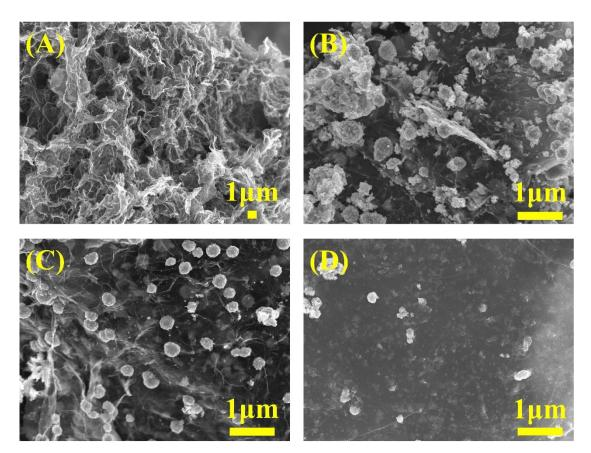
Fig. 2. SEM images of different counter electrode materials: (A) RGO, (B) Co/RGO0.05, (C) Co/RGO0.1, and (D) Co/RGO0.5
