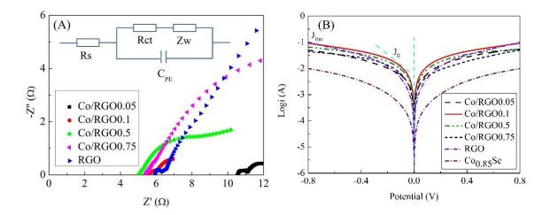
Fig. 4. Electrochemical properties of different CEs, EIS (A), and Tafel polarization curves (B) (color online)
