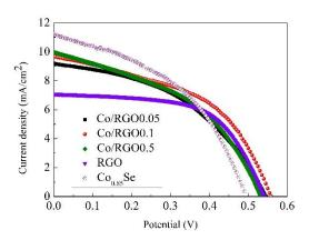
Fig. 5. Current density-voltage (J-V) curves of different QDSSCs assembled with CdS/CdSe co-sensitized TiO<sub>2</sub> photoanode,  $S^{2-}/S_n^{2-}$  electrolyte, and different counter electrodes (color online)
