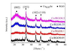
Fig. 1. XRD profiles of prepared Co<sub>0.85</sub>Se/RGO composite CEs (color online)
