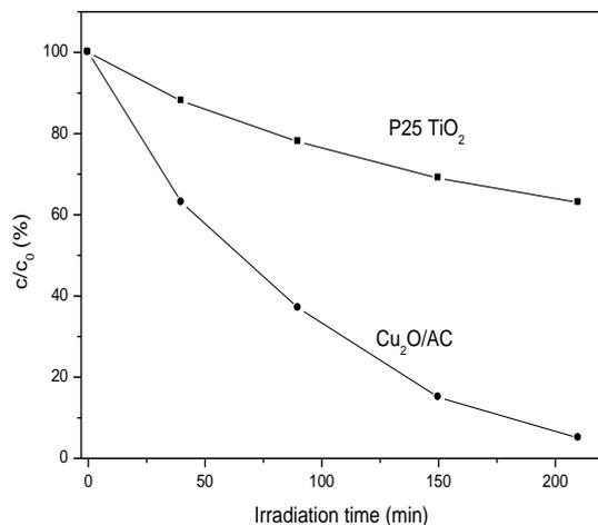
Fig.3 Photocatalytic activities of different photocatalysts under visible-light irradiation.
