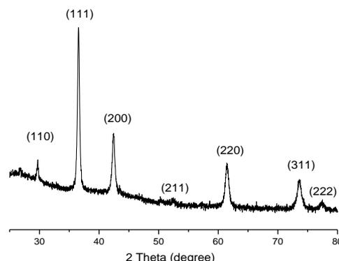
Fig. 1 XRD pattern of  $\text{Cu}_2\text{O}/\text{AC}$ .
