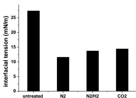
Fig. 3. Interfacial tension with blood and tissues of PVDF films untreated and treated in a microwave plasma with different discharge gases.
