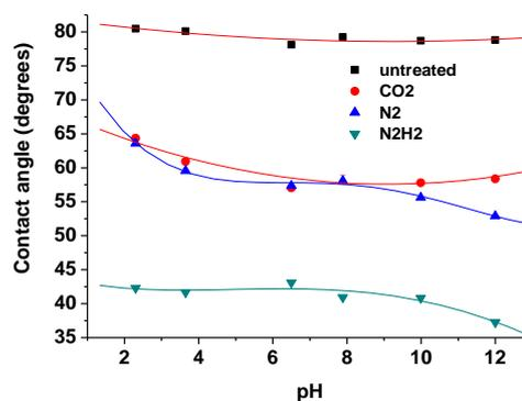
Fig. 5. Variation of the contact angle with pH for PVDF surfaces treated in microwave plasma of different gases.
