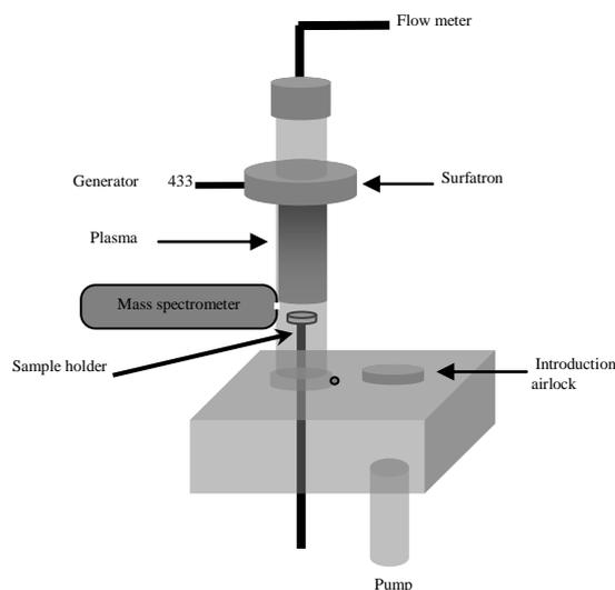
Fig. 1. The experimental set-up for plasma treatment of the PVDF surface.
