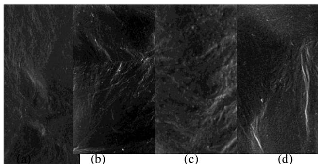
Fig. 7. SEM images of the PVDF substrate as reference (a), and treated in the optima microwave  $\text{CO}_2$  plasma conditions (b) and grafted with protein A (c) or triglycine (d) after  $\text{N}_2$  or  $\text{N}_2/\text{H}_2$  microwave plasma treatment.
