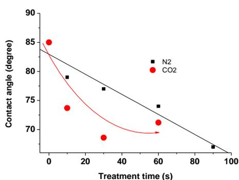
Fig. 2. Contact angle between water and the PVDF surface plasma treated with different gases.
