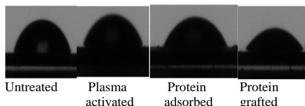
Fig. 4. Contact angle images of the plasma exposed surfaces and subsequent coated/grafted with proteins
