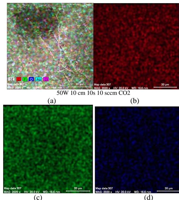
Fig. 9. EDX cartographies of entire composition (a) and in carbon (b), fluor (c) and oxygen (d) for PVDF. Film surface treated by  $\text{CO}_2$  plasma.
