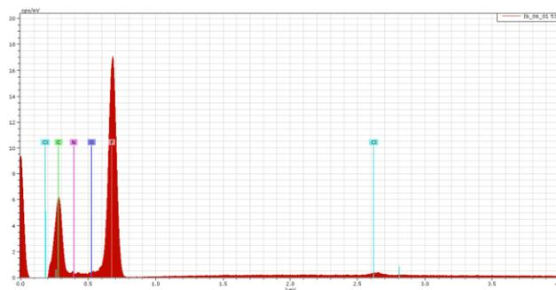
Fig. 8. Typical EDX spectra of the PVDF film surface
